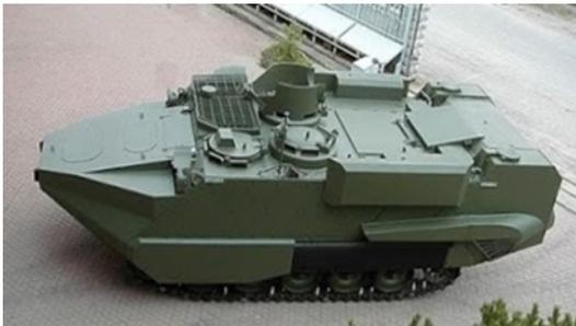
(80) Arisgator M113s - fielding 12.7mm guns, 40mm grenade launchers, with mortar and ATGW variants.
