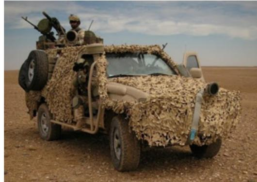
(5000+) Hilux Technical Vehicles - will be fitted with armoured windscreens and ballistic protection inserts around the cab and engine to protect against 7.62mm rounds. They will be armed with 12.7mm guns and ATGWs with (standard) high magnification sights, plus some vehicles will carry 81mm mortars.
