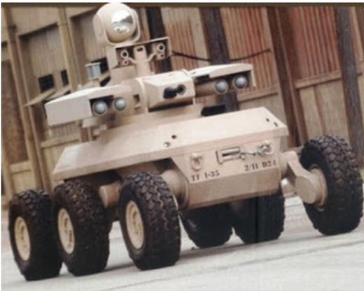
(100+) Wheeled Autonomous Robotic Vehicles - to be used as convoy lead vehicles in the anti-mine role and as gun platforms using 12.7mm weapons and ATGW.
