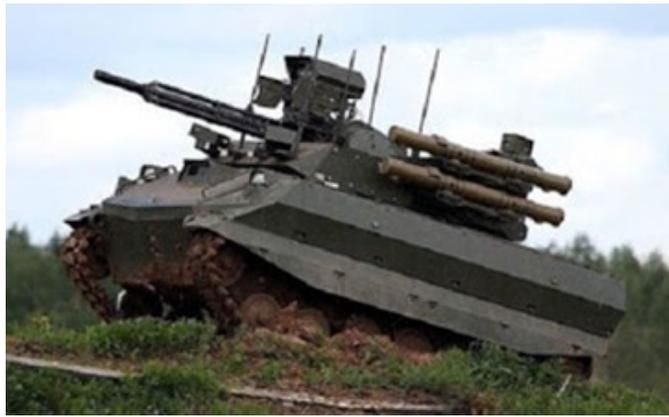
(50+) Uran-9 tracked UGVs - will be trailer mounted for transport and equipped with a 30-40mm gun and ATGW.
