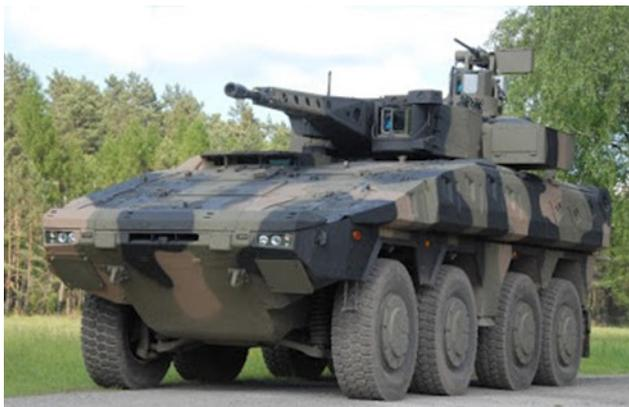
350+) Boxer CRVs to act as the leading rapid reaction force vehicle, functioning as Armoured Scout-IFVs (fitted with twin ATGW launchers), 105mm/120mm turret Fire Support/Anti-Tank, 120mm Mortar, AAA, Command, plus Evac roles.
