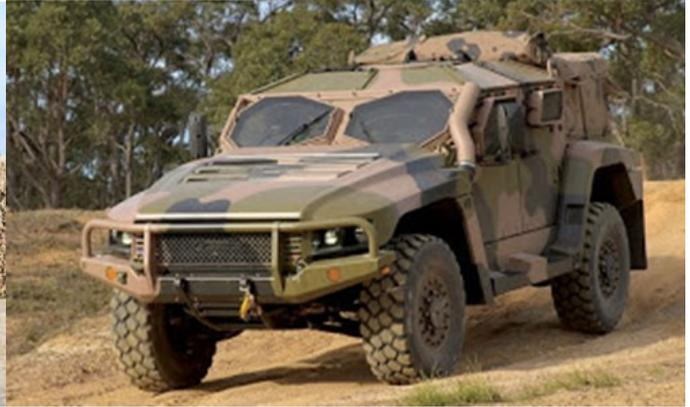
(1100) Hawkei LPMVs for scouting & light utility, upgraded with engine compartment protection against 7.62mm rounds, and featuring weapons options available to the VBL or L-ATV.
