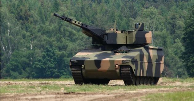
With an assumed turbocharged diesel-fueled engine serving as its powerpack, the vehicle has an estimated road speed of 70 kmh (this falls to 40 kmh when going cross-country) and an operational range nearing 500 kilometers.
