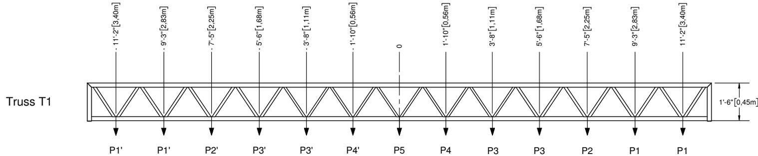
$$\text{Truss T1**}: \frac{\text{Load P1}}{\text{Capacity P1}} + \frac{\text{Load P2}}{\text{Capacity P2}} + \frac{\text{Load P3}}{\text{Capacity P3}} + \frac{\text{Load P4}}{\text{Capacity P4}} + \frac{\text{Load P5}}{\text{Capacity P5}} \leq 1.00$$
