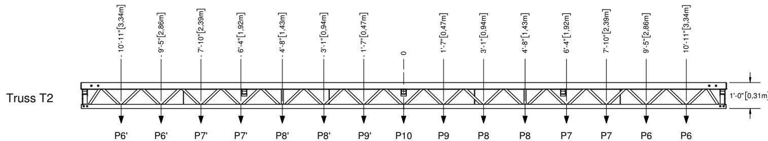
$$\text{Truss T2**}: \frac{\text{Load P6}}{\text{Capacity P6}} + \frac{\text{Load P7}}{\text{Capacity P7}} + \frac{\text{Load P8}}{\text{Capacity P8}} + \frac{\text{Load P9}}{\text{Capacity P9}} + \frac{\text{Load P10}}{\text{Capacity P10}} \leq 1.00$$
