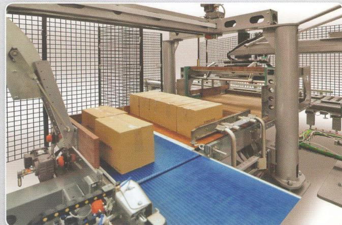
Roller conveyor pre-formation composed of a powered carpet: packs are stopped in the right position thanks to a changing of the carpet speed. Both a pack spacing unit and a pack-turner are included, too.
