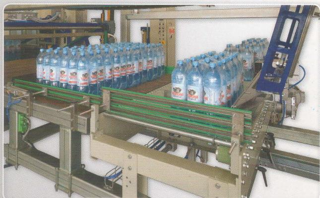
The palletizers are manufactured with a double-column frame, they are checked by PLC which, in case the machine should be supplied with the accessories, it guarantees quick and automatic formats change-over.
