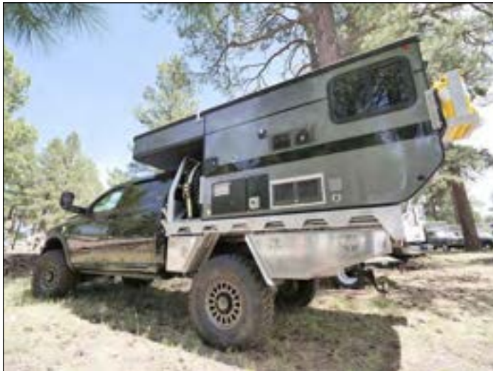
Large 37x12.50R17LT Goodyear Wrangler MT/R is only a 50psi tire, but the tire volume makes the SRW rating 3,525-lb each. I prefer the handling attributes of higher psi tires.
