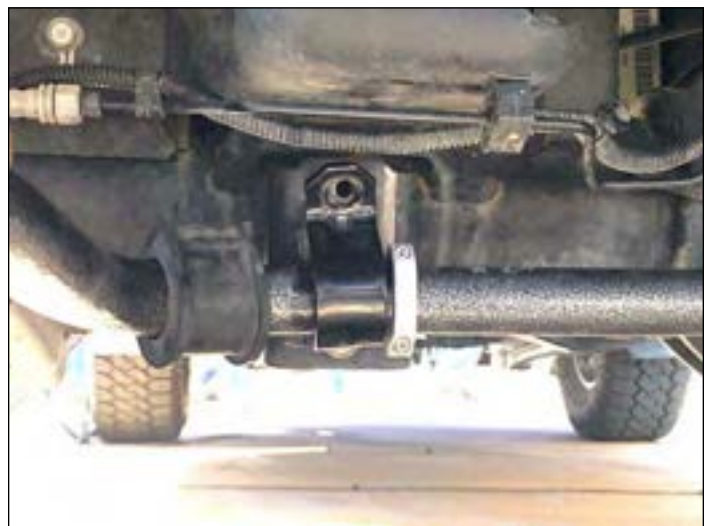
Missing bolt and bent Hellwig Big Wig rear stabilizer bracket explained the loose handling.
