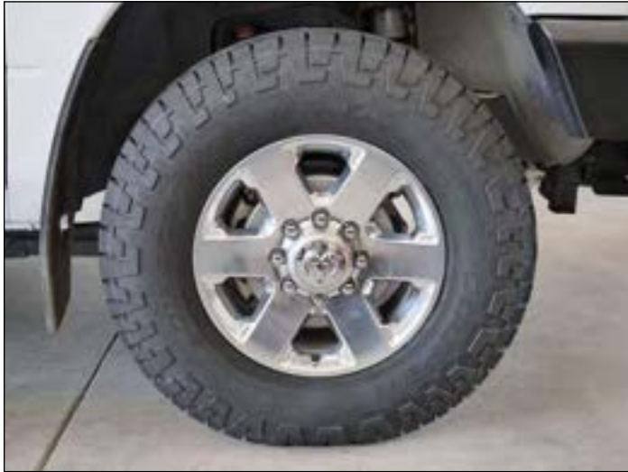
Cooper's AT3 XLT in 285/75R18E (34.84") with a 129 load index can handle 4,080-lb each at 80psi.
