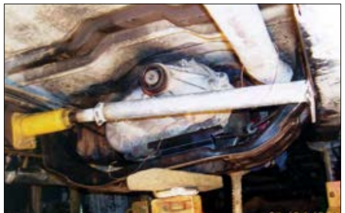
Troy Simonsen's bottle jack/pipe extension trick to spread the frame rails from Issue 68, page 13.
