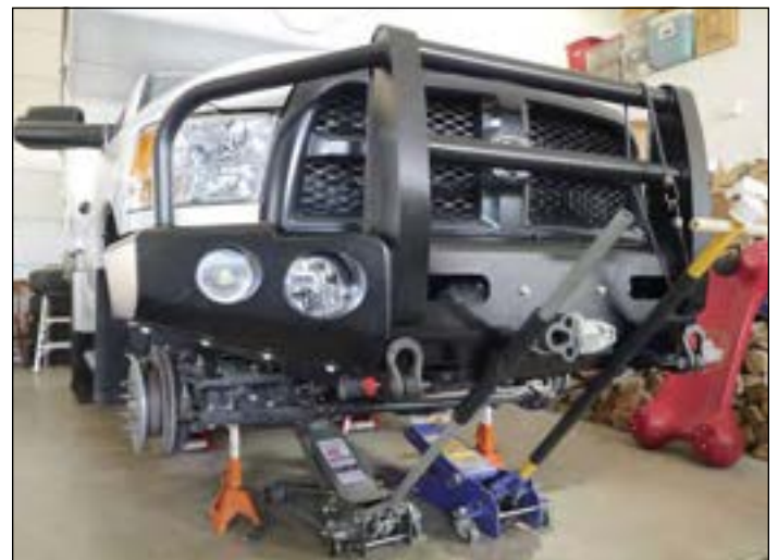
Two 6-ton jack stands support the frame and truck, floor jacks allow controlled axle droop, and smaller jack stands under the axle for backup.
