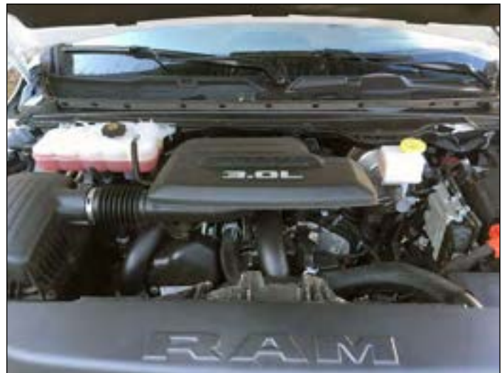
Under the hood is the third generation of the 3.0-liter VM “EcoDiesel” engine. The first was VM’s A630 for the European market. The second was the L630 for the 2014-2019 U.S. market. Details are in Issue 106, pages 20-21.
