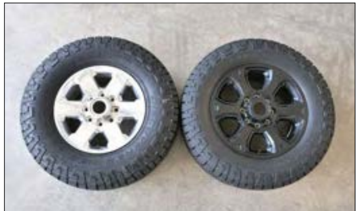
18" wheel on the left, 20" wheel on the right, all other specs are very similar.
