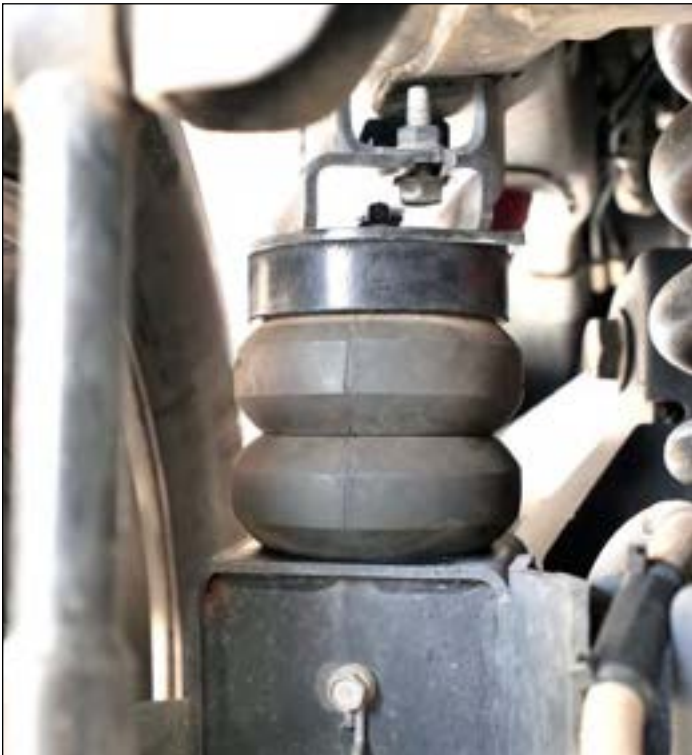
The rear axle load sitting on the Aeon double-convoluted rubber spring with the 1" spacer added.
