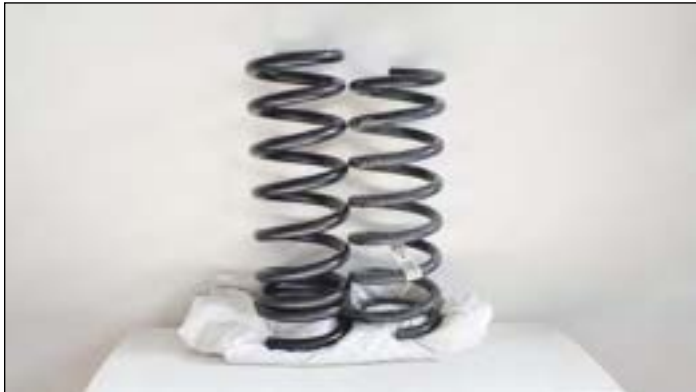
TufTruck TTC-1224 on the left, taller and made with larger wire diameter than the OE spring on the right.
