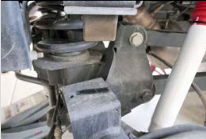
The clean spot atop the rear axle indicates the OE bump stop had made contact.
