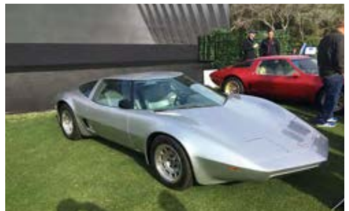
Here is the 1973 "Aerovette," a mid-engine concept car with a rotary engine.
