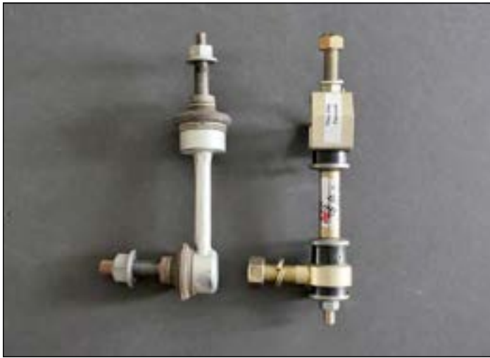
Stock front sway bar link next to replacement SuspensionMAXX end-link from Geno's Garage.
