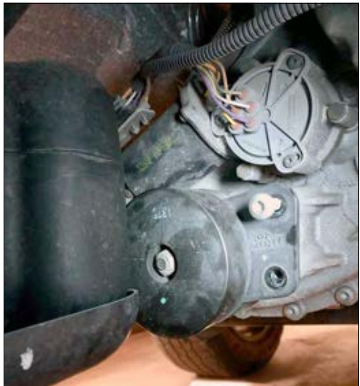
The drain plug is behind the harmonic/vibration counter weight. Inconvenient: yes.
