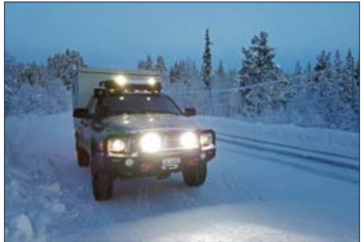
A cold weather test of the camper "Box Two." The first camper allowed ice build-up on the interior storage compartments.
