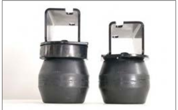
Timbren DRTT3500E single-convoluted spring kit, shown with the included 1" spacer on the left, and without on the right.
