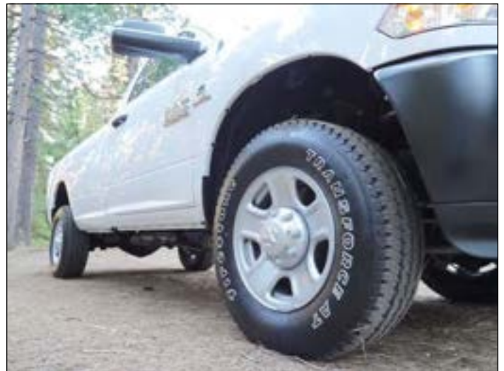
People don't complain about the stock 275/70R18E having a short sidewall. SRW capacity is a respectable 3,640-lb at 80psi.
