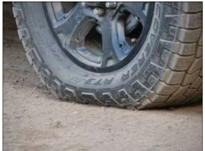
Shorter 20" sidewalls are a bit less forgiving at full psi on the roughest roads, lowering pressure helps. This Cooper AT3 XLT 285/65R20 was initially tested at 37psi, but is at 30psi in this photo. Dropping the extra 7 psi was a big improvement.
