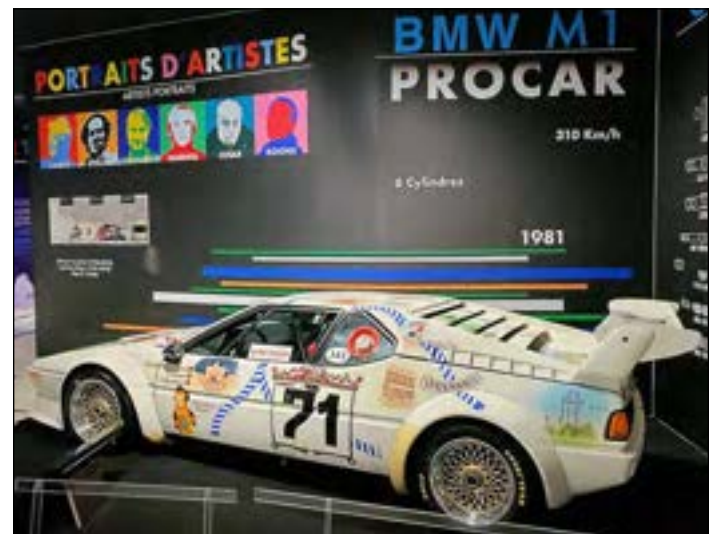
Another car on display at the LeMans museum, the BMW M1. A highly tractable straight-six engine contributed to the 1981 BMW M1 ProCar's racing prowess, gracing it with 470hp and a top speed of 193mph.
