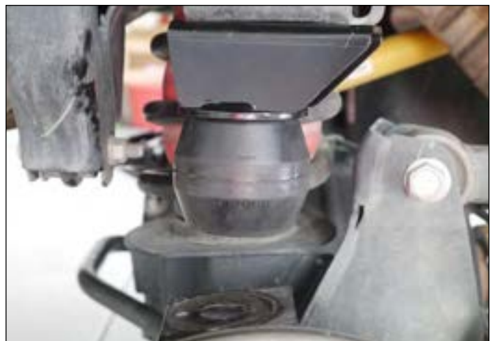
These Timbren DRTT3500E replacement springs are quick and easy to install.
