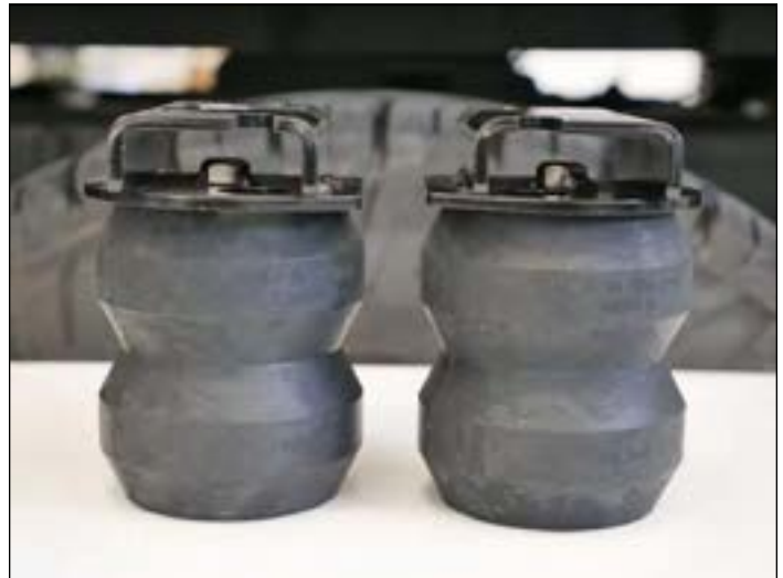
Timbren DR2500D rubber auxiliary Ram 2500 rear springs kit.
