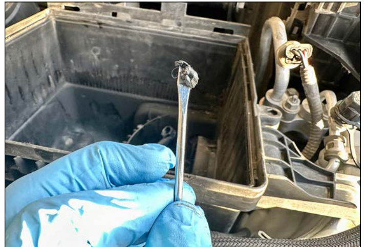
Oily grit scraped out of the air-box.
