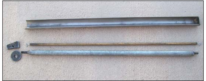
Camshaft changing tools. Trough for tappets at top, fulcrum and plates that clamp to cam gear on bottom.
