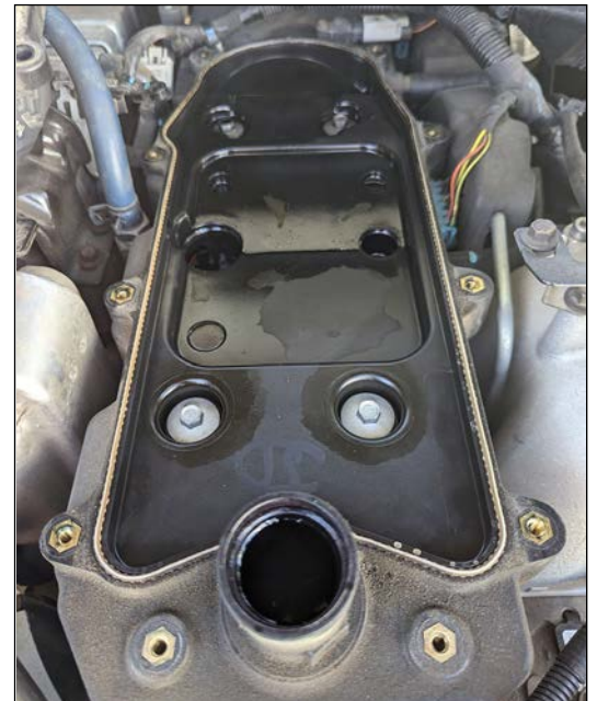
This is actually the valve cover. Just check the white perimeter gasket for condition. Wipe it clean, lube the O-rings with some oil and press the new filter in place. Reinstall the cover and torque the bolts and studs to 89-inch pounds.
