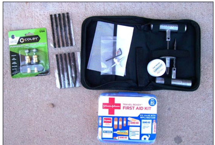
Colby tire valves top left, tire plugging ropes and kit with tools to install rope and ream hole in tire to the right. First aid kit on the bottom.
