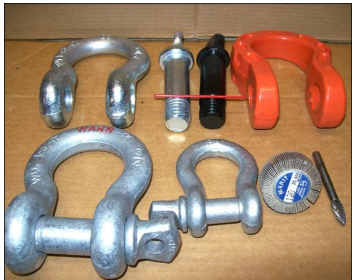
Steel shackles showing forging roughness, bottom left and center. Polished shackles top left and right, with pins top center. Carbide bur and polishing wheel bottom right.
