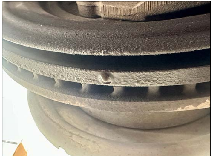
Gear oil dripping from a brake rotor.
