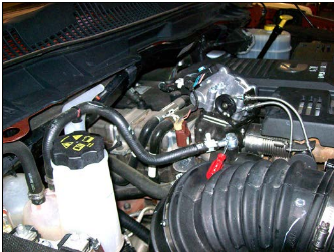
Banjo bolt to loosen for purging air from the cooling system.
