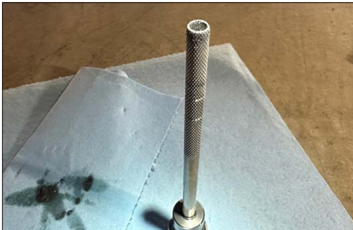
It seemed wise to check the rear axle oil level after a leak. It was fine. No shavings or material to speak of on the magnet in the tip of the Mag-Hytec dipstick.
