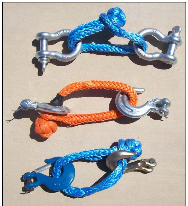
Three attachment positions for soft shackles—central, behind the knot, and at the loop.
