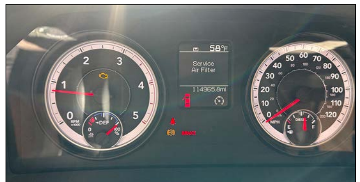
Service Air Filter warning on my Tradesman EVIC, which was accompanied by a warning bell that continued to chime every few minutes. The Edge Insight scanner showed code P2280, intake flow restriction. The Edge Insight was then used to erase the trouble code.
