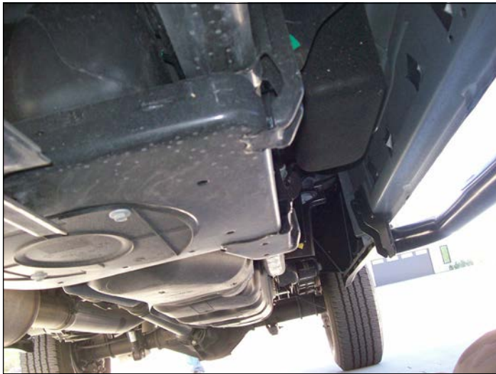
50-gallon fuel tank on his Turbo Diesel.
