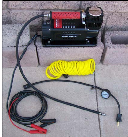
Maddox air compressor, top. Yellow extension hose, center. Power cables in lower left, and hose with integral pressure gauge lower right.
