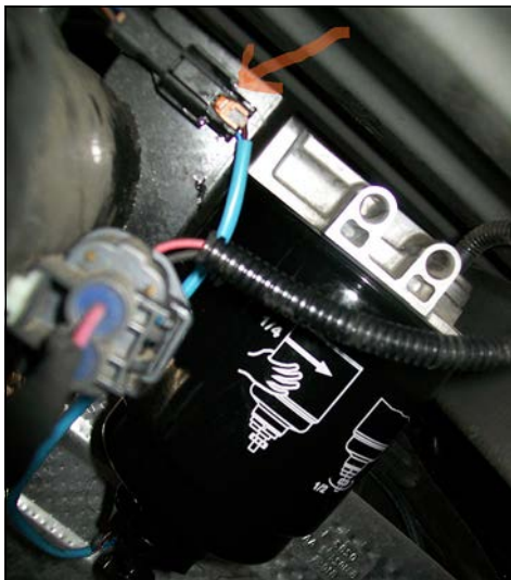
Chassis mounted filter with water-in-fuel sensor connection at top, painted orange.
