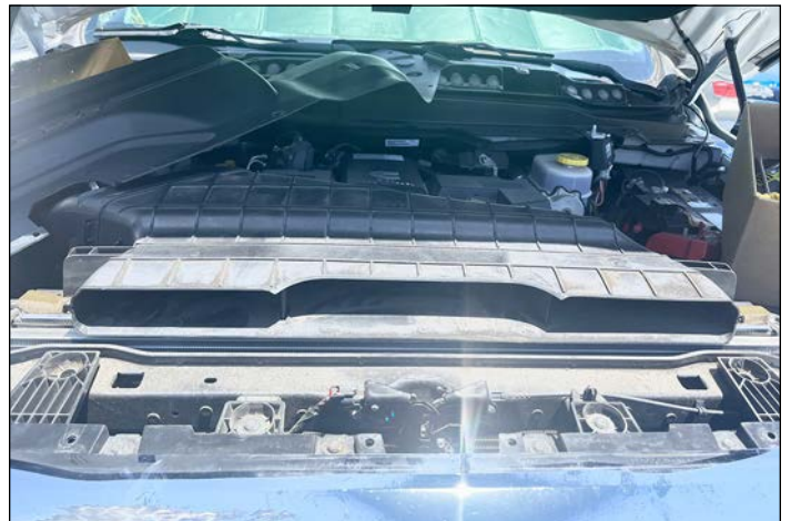
Editor's truck: The 2019 and newer trucks: Air ducting from the top of the radiator/lower lip of the hood.
