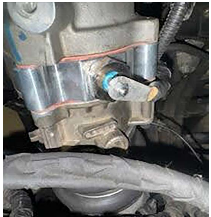
Black Market Performance Grid Heater Relocation Kit. It is installed between the air horn and cold CAC pipe. Notice the red gasket above and below the spacer. It acts as a perfect insulator so unless one of the mounting bolts is touching the spacer to provide a ground path, the heating element will not operate.
