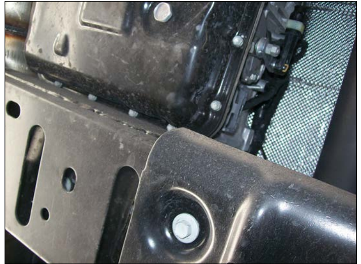
Aisin crossmember still restricts access to the pan bolts.
