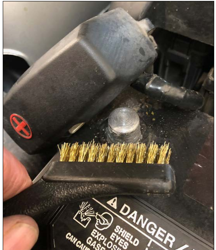
Wire brush for clean-up of battery terminal(s).
