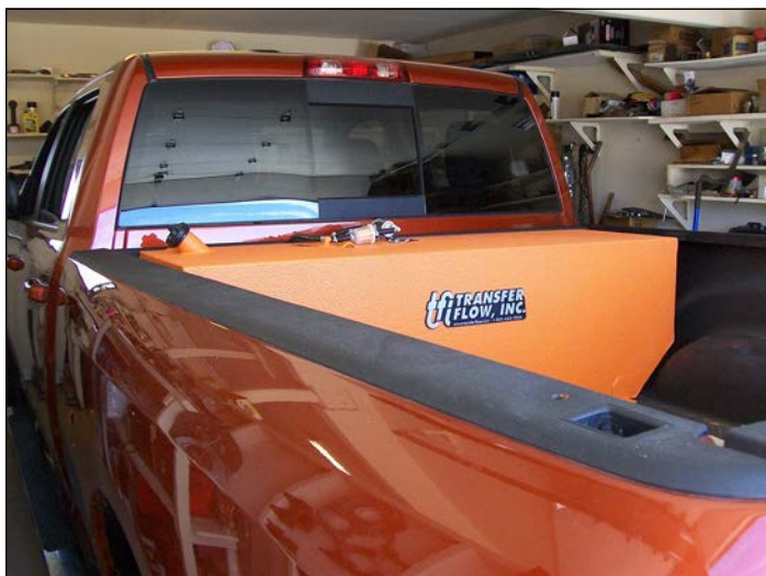
75-gallon Transfer Flow tank installed in my 2013 Ram.
