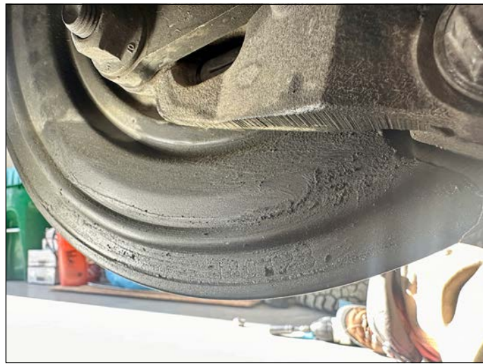
Backing plate still had some caked-on dirt after the repairs.
