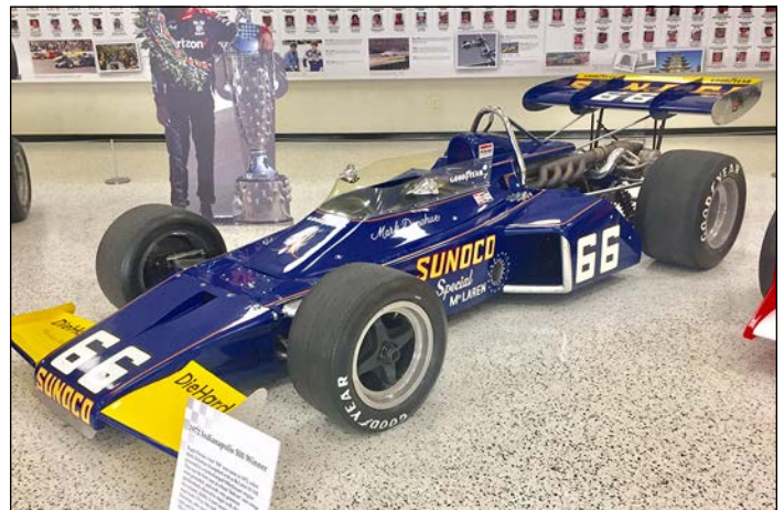
1972 Winner, Mark Donohue. Big wing in back equals downforce, equals a speed differential of 18mph faster (195mph versus the previous 178mph). (Indianapolis Speedway Museum 2019)
