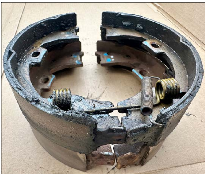
Parking brake shoes and hardware are not supposed to be oil-soaked.
