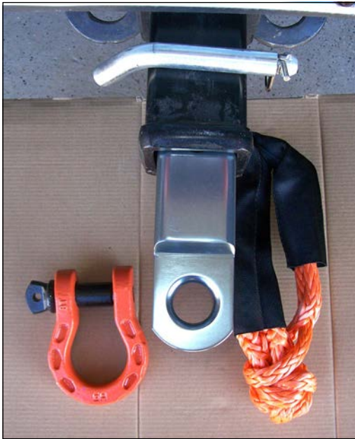
Recovery point for trailer hitch with steel and soft shackles.
