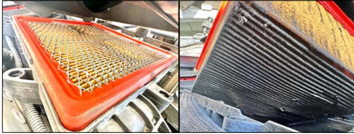
Top of the filter looked just fine. Lifting the filter out of the air-box told the story!
