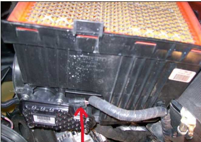
Side of the air box facing the engine, with red arrow to the electrical connector.
