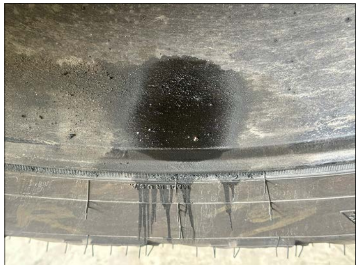
Oil was also inside the wheel and showing traces down the tire sidewall.
