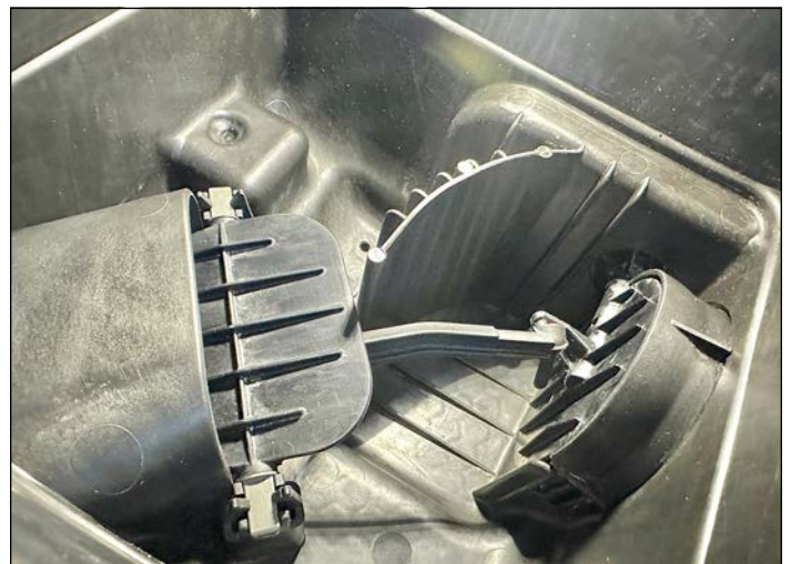
Almost as clean as new. Ram-air actuator reconnected.
