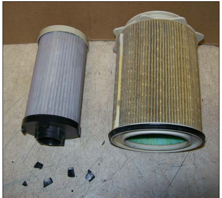
Used engine mounted fuel filter with central core removed. How do the filter(s) look to you?
