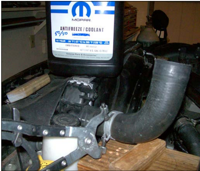
Filling the radiator and engine with coolant using an elbow shaped piece of radiator hose.
