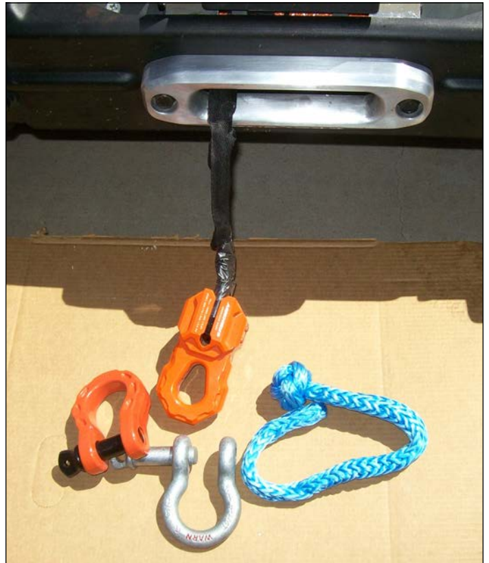
Hawse fairlead at top, with winch line to Agency 6 closed shackle that can accommodate steel shackle pin, shackle body, and soft shackle.
