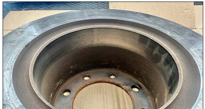
What the surface and interior of a brake rotor should look like. (This was the "good" left side.)
