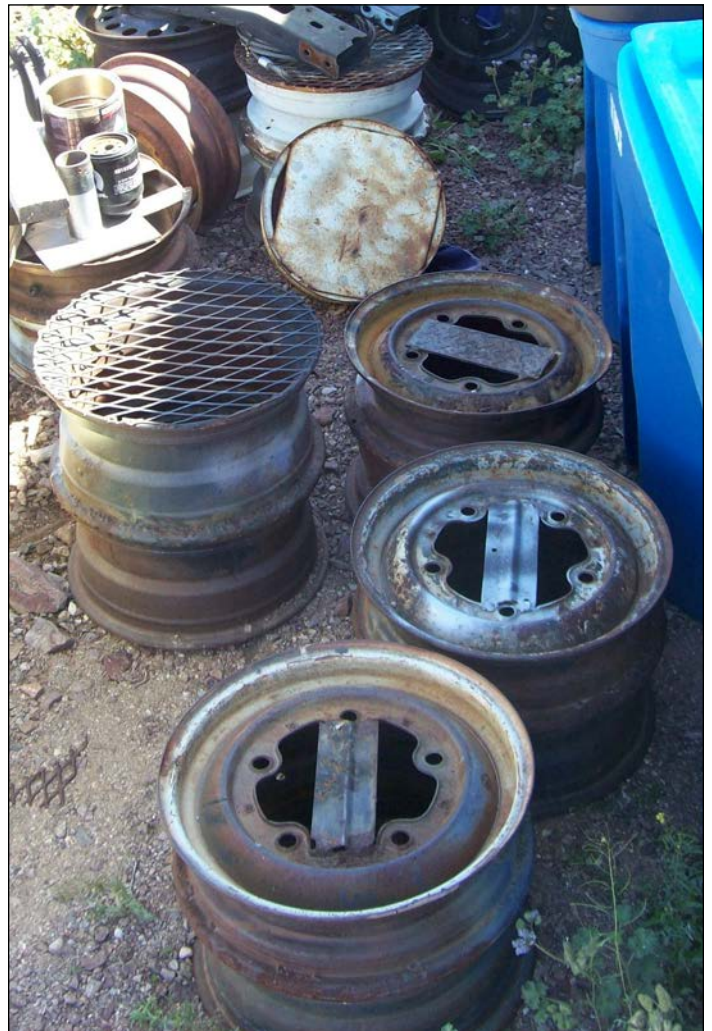
Different height welded wheels to use as stools and as jack stands.
