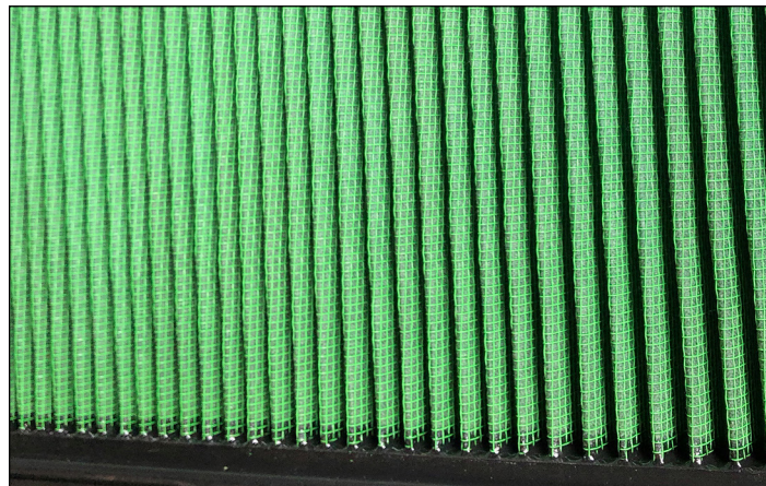
Green Filter's filter border (black) meets media area with a clean-cut line. Nice manufacturing.
