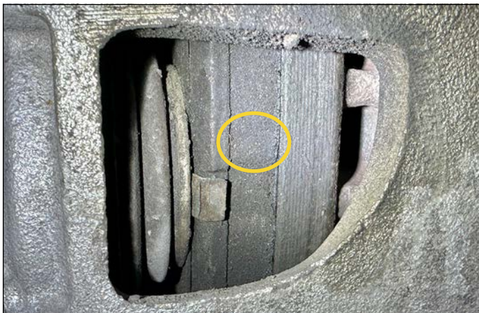
Impressively thick brake pads after 100,000 miles.
