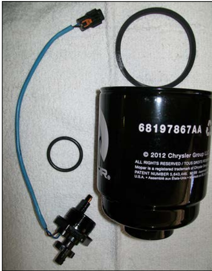
Turbo Diesel rear, chassis mount fuel filter with water-in-fuel sensor at the left.
