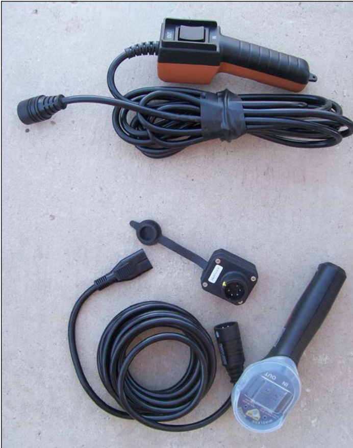
Conventional winch controller at the top. Below is a remote controller, with module for the winch control box and an auxiliary power cable for the remote in case of battery failure.
