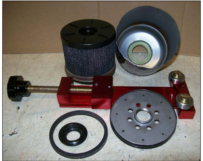
Used chassis mounted fuel filter that was cut open with an oil filter cutter.
