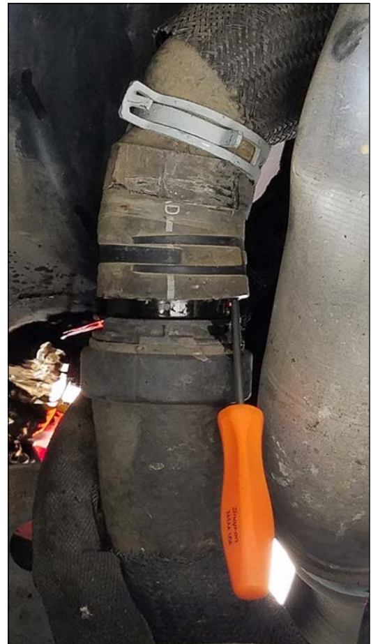
Connection for draining coolant on 2015-18 Turbo Diesels.
