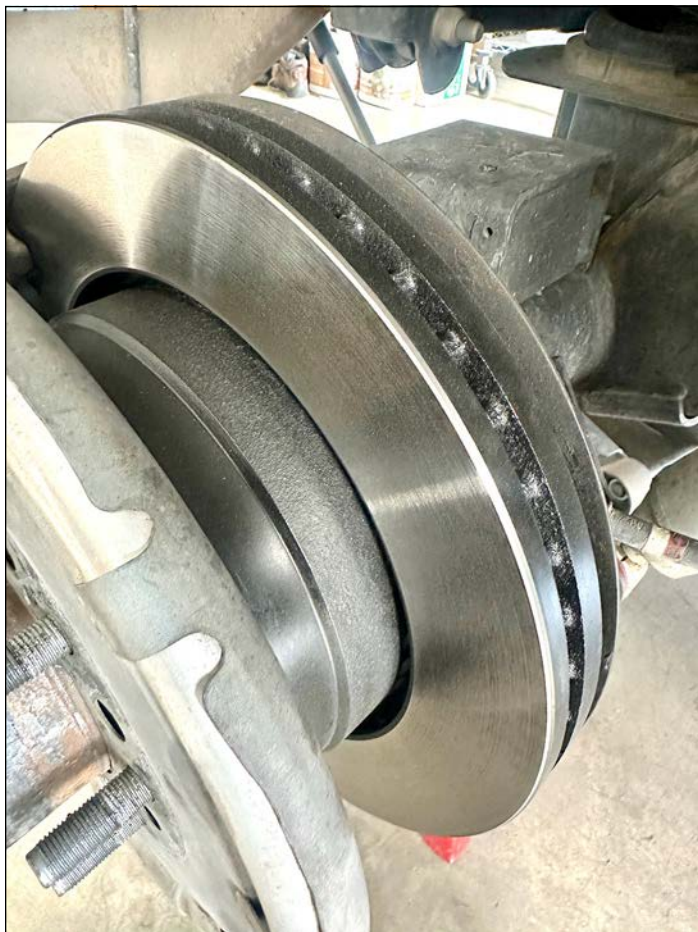
Raybestos part #780733 rotors for the rear axle.
