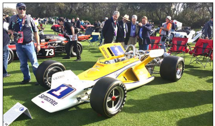
This car was designed to race at Indianapolis in 1972 with "dihedral" wings. There was not enough time for development and they were removed. (Amelia Island 2018)
