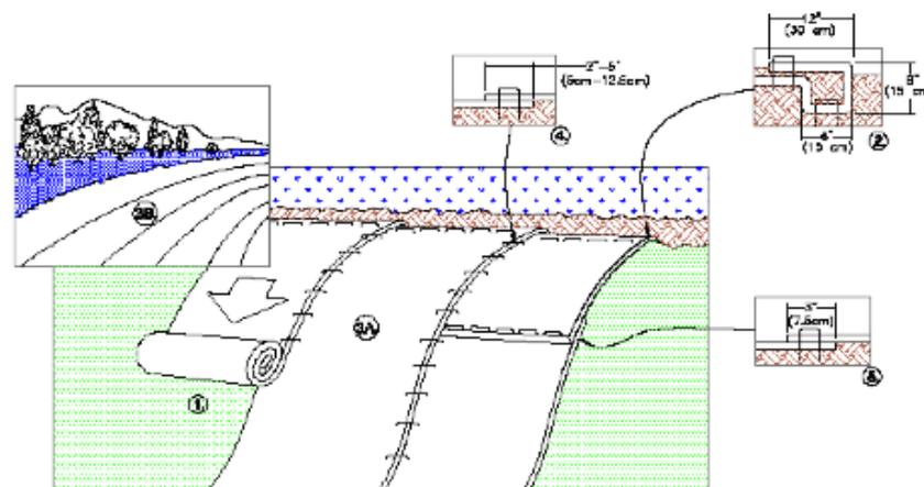
1. PREPARE SOIL BEFORE INSTALLING BLANKETS, INCLUDING ANY NECESSARY APPLICATION OF LIME, FERTILIZER, AND SEED.
