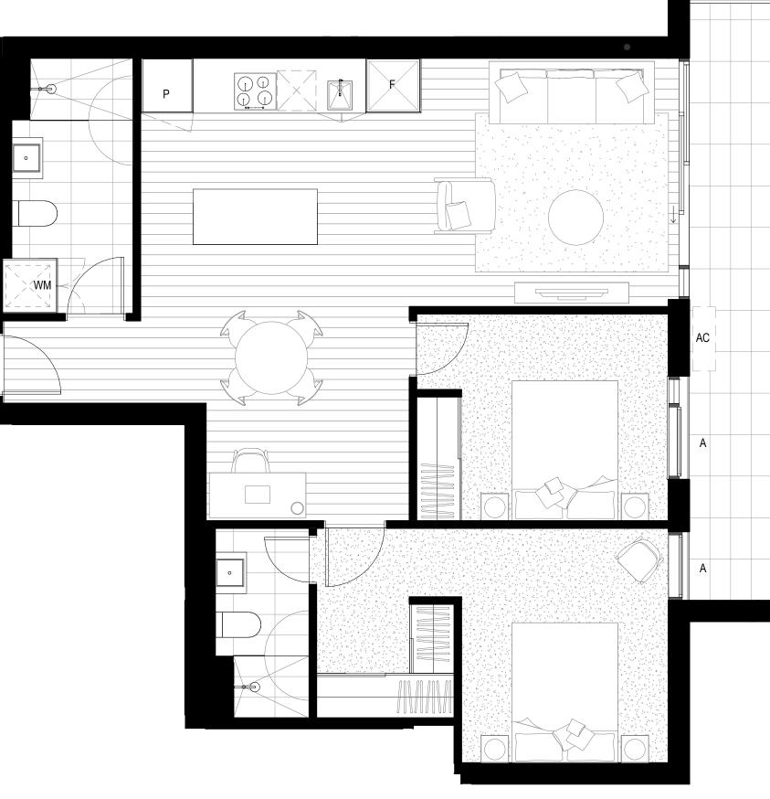
P: PANTRY LN: LINEN CUPBOARD F: FRIDGE WM: WASHING MACHINE AC: AIR CONDITIONING CONDENSER A: AWNING WINDOW
