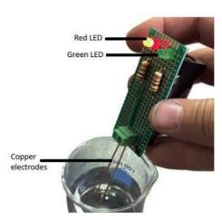
The meter has a 9V battery, two parallel copper electrodes and
