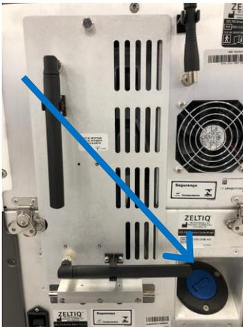
2. Press down on the recessed end of the blue lever on the chiller tank cap.
