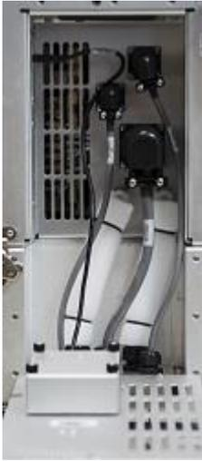
3. Working from left to right, disconnect the cables and then the hoses.
