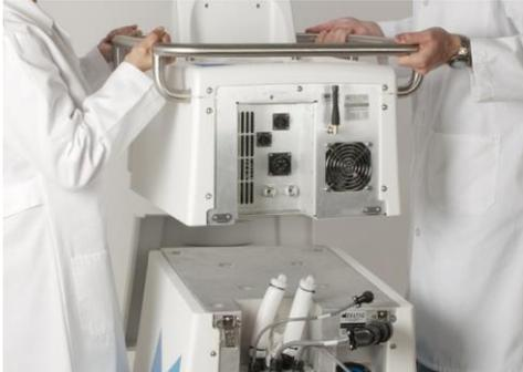
6. Walk past the base module and put the upper module down.
