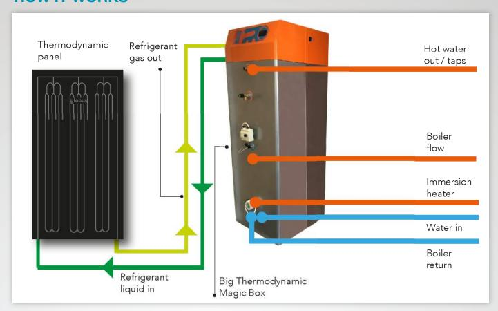
The Thermodynamic Collector circulates refrigerant liquid where energy is absorbed from the ambient temperature.
