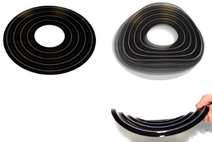
Figure 12. Transformation from a Flat 4D Printed Structure to a Curve-Crease Origami Structure Approximating a Hyperbolic Paraboloid [14]
