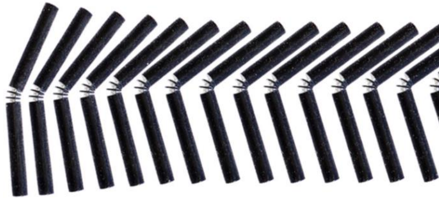
Figure 9. 4D Printed Joints Showing Custom Angles [14]
