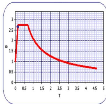
Graph 1. Building response verses fundamental structure period of vibration in ferrocement reinforced concrete shear wall
