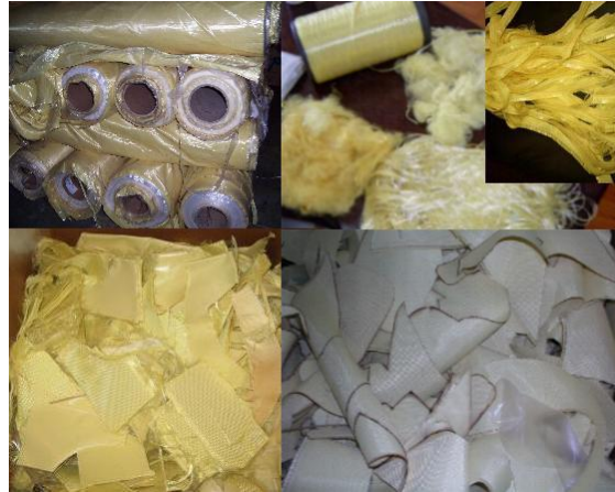
Figure 21. Kevlar chopped and ready to be recycled.
