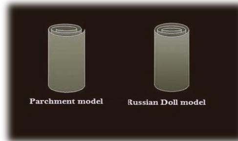
Fig. 1. Structural Rolling Graphene sheet methods (Etemadi, A. 2014).
