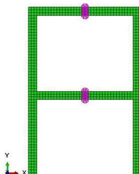
Figure 8. The spring element for two divided parts of the model
