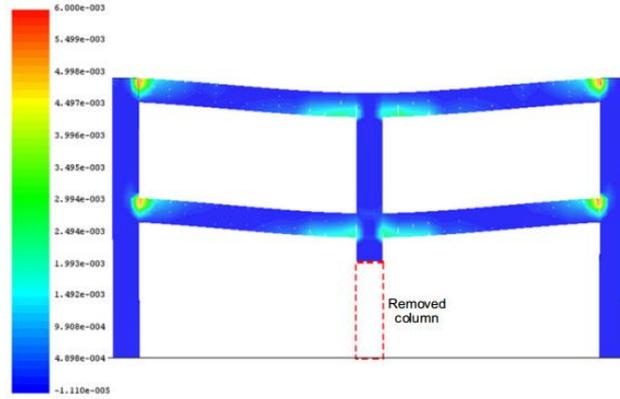
Figure 9. Principle strain contours after internal column removal (Huda Helmy et al. 2012)
