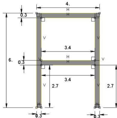
Figure 1. The geometry of RC structure.
