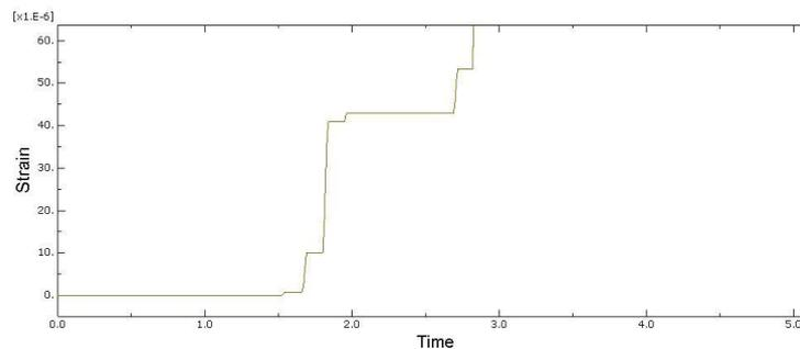
Figure 14. Plastic strain graph in the column-beam connection in the first floor for model 2
