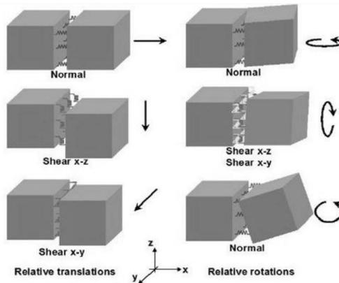
Figure 2. The spring element in AEM.
