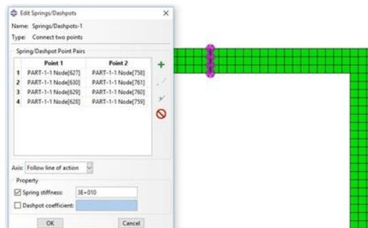
Figure 7. Spring element properties in AEM model.
