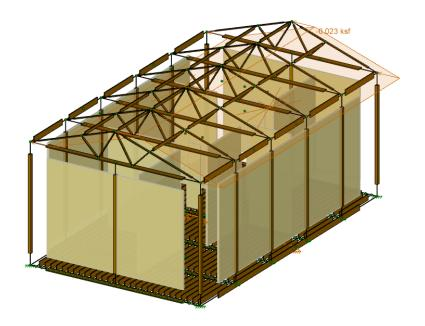
This picture shows the structure from the underside. I have my joists pinned connected to my beams, and my beams pin connected to my columns. Through research, I decided to space my joists 1' apart due to common practice. This design provides equal load distribution to the ground.
