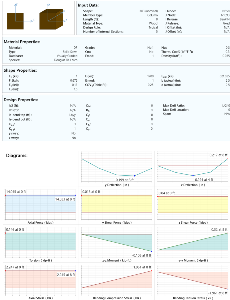
Figure 22. Data collected from wooden stud in the attic.
