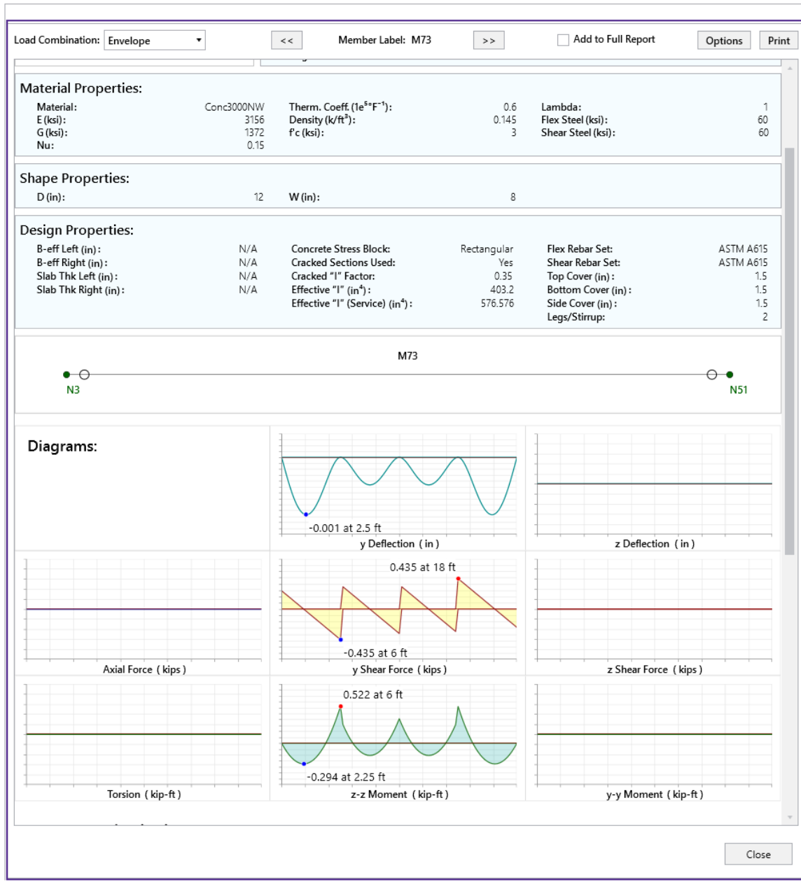
Figure 4. Structure report of one of the concrete beams under the five columns
