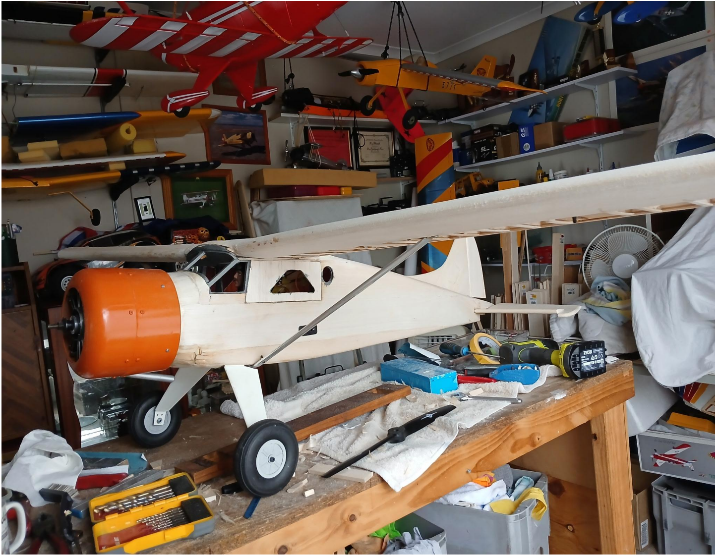
Above – Rex has been busy and is almost ready to cover his DHC Beaver. It has a 71" wingspan and a Saito 82 engine
