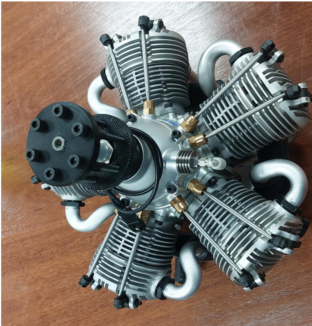
Above - Fred showed this new 150cc 5 cylinder Radial Engine at the meeting
