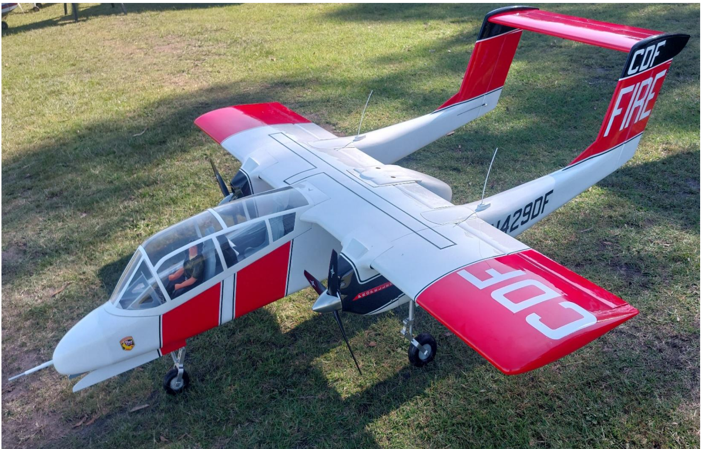
Above - Fred's Hangar 9, OV-10 Bronco - 84" span, 2 x 20cc 6S electric equivalent motors.
