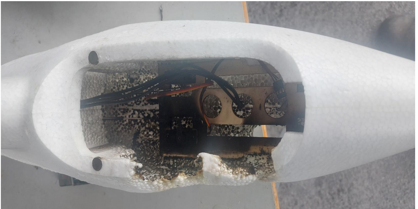
Above and below – This is the result of having the throttle on when the model is on the ground....upside down. a melted ESC and melted foam fuselage. Bad Luck Doug
