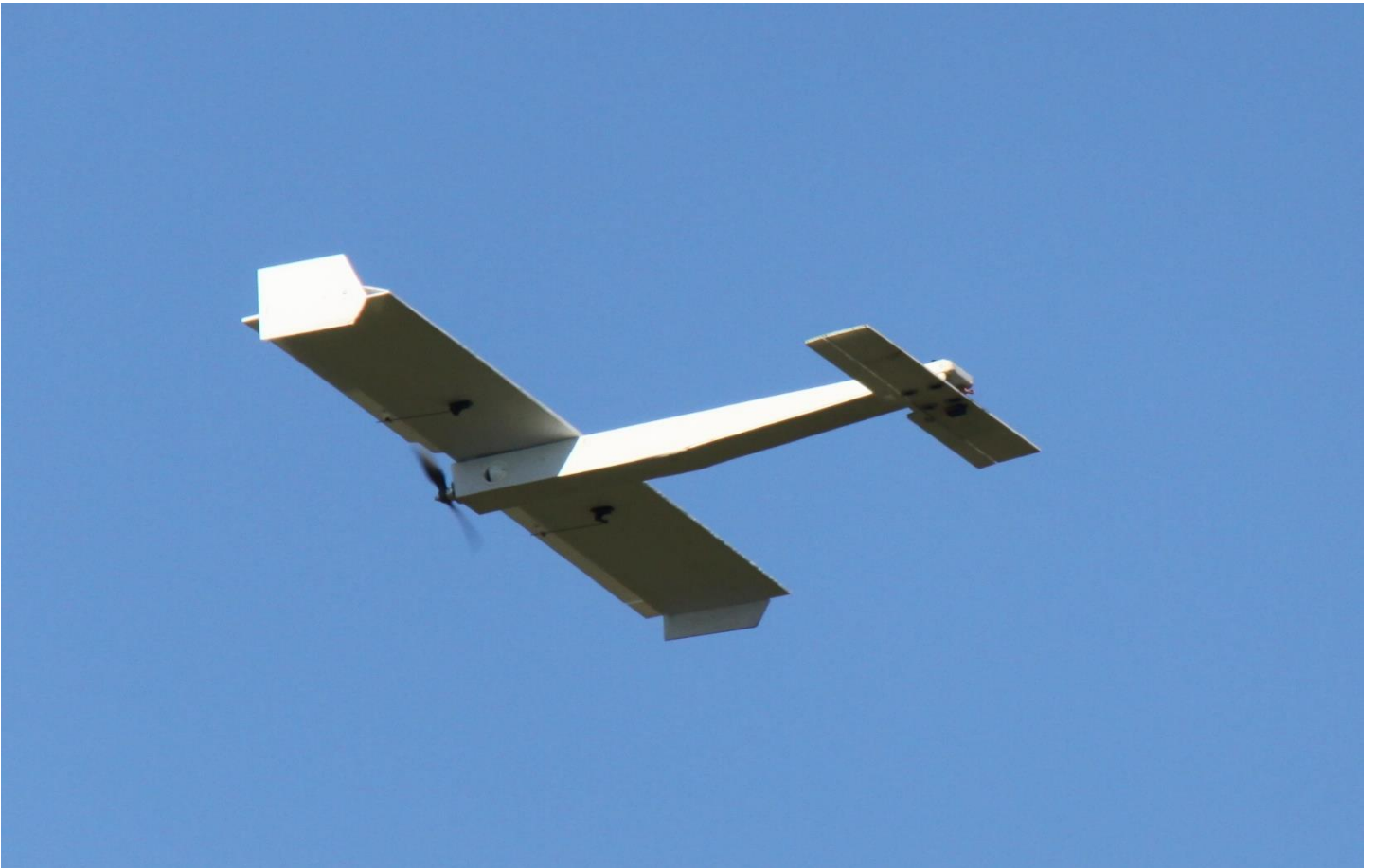
Above – Lofty's Canard – they fly quite well – He has fitted an undercarriage but it doesn't handle well on the ground
