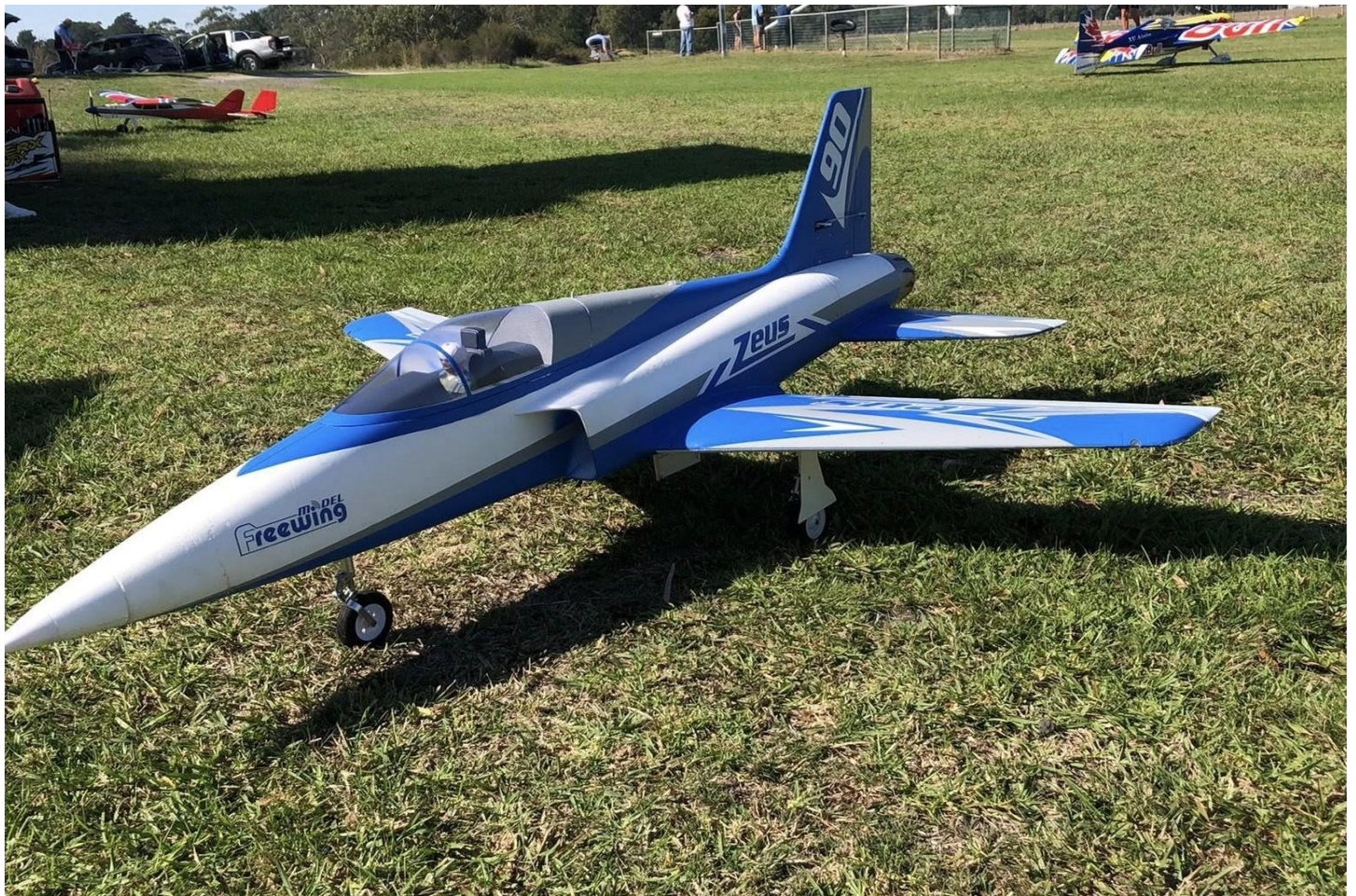
Above – Jamie McLaughlin is flying this very nice Zeus Jet, running on a 90mm EDF You can buy a kit to convert this Foam Jet from the EDF motor to a Turbine.
