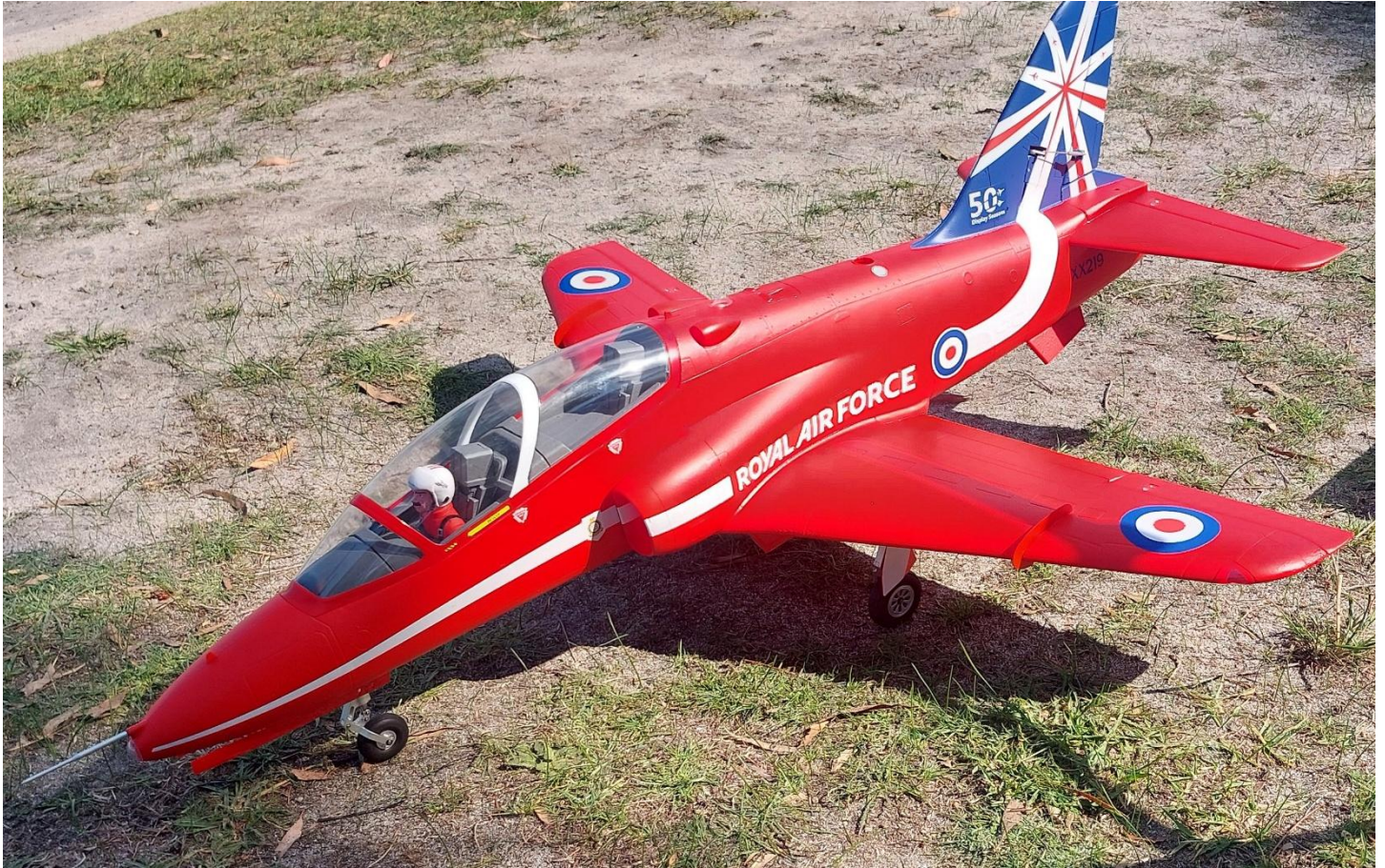
Above – Craig has a new Jet – The FMS BAE Hawk –80mm Fan, 100Amp ESC, 6S Battery – Fly's very well & sounds great
