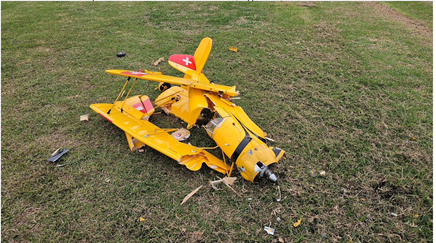
Rex has had this nice scratch built "Jungmeister" for some years but it didn't make it home in one piece on this day. Paul's postmortem revealed a failed elevator servo (stripped teeth) caused it to hit the deck.
