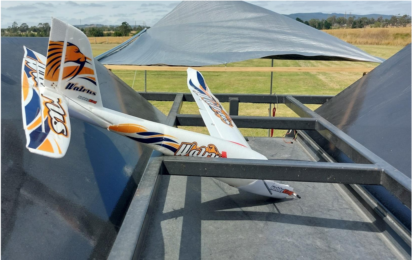
Above – Jamie's Walrus crashed into the middle of Wayne's trailer after a launch with a faulty aileron servo
