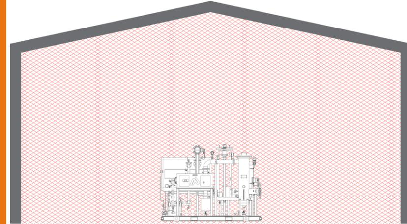
This room is continuously ventilated at 12 air exchanges per hour.
