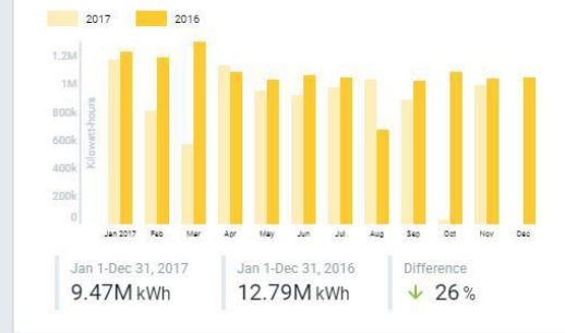
Amway Center's Electricity Use Post LED Retrofit Last 12 months
