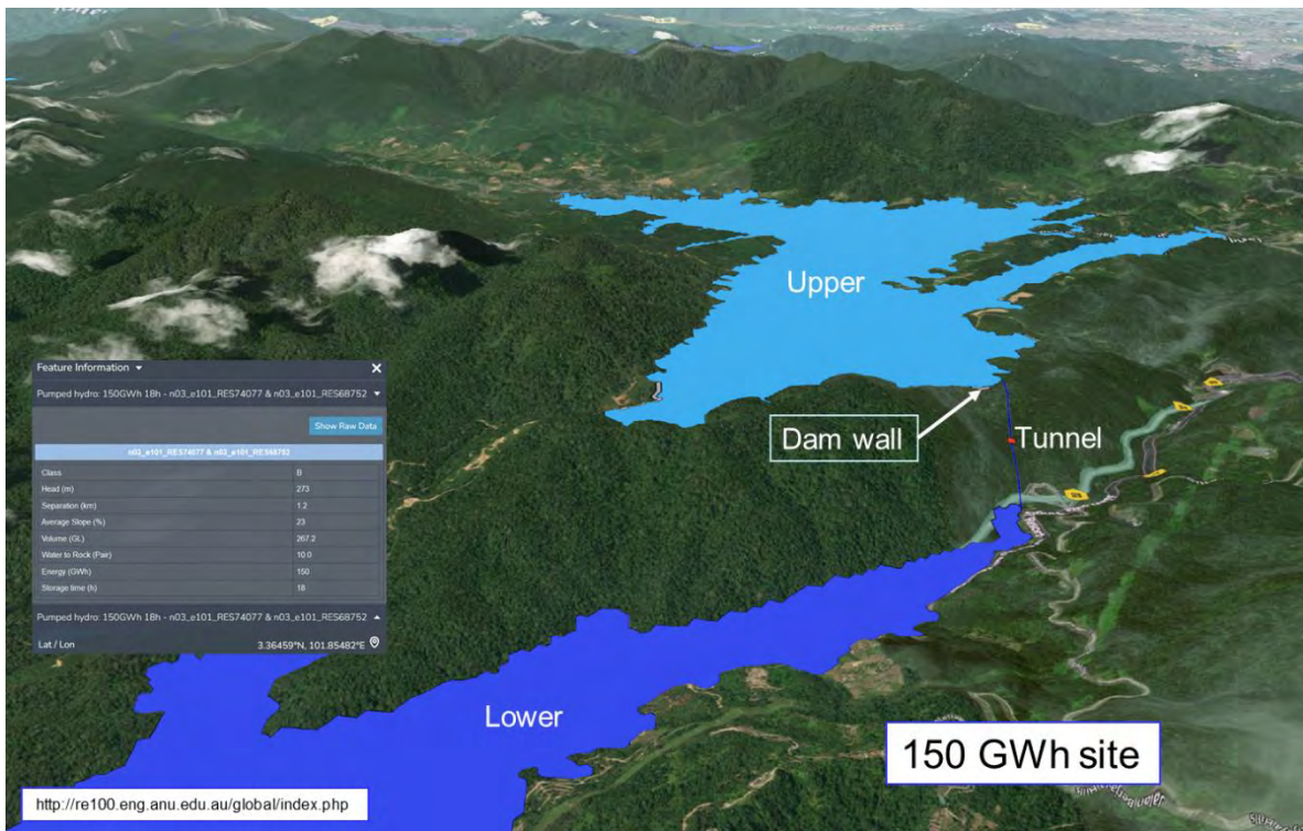
Figure 8: Greenfield – detail of one of the 616,000 STORES sites we found worldwide including information popup.
