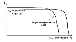
Because  $I_O$  is temperature dependent, the open-circuit voltage drops with temperatures. Through one end of a p-n junction, the formula is;
