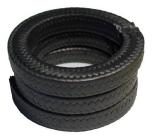
Packed Seals use a soft woven lubricant infused yarn (the most common of which is graphite impregnated Teflon) pushed up against the pump shaft and pump housing by a bolt tightened gland follower. A small amount of liquid is allowed to leak through this assembly to provide a fluid film for lubrication and heat rejection. A rule of thumb is that 10 to 50 milliliters a minute per inch of shaft length is usually sufficient for this purpose.
