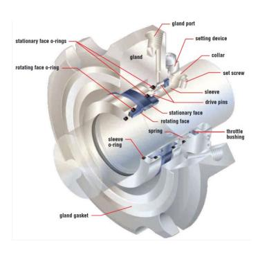
Mechanical Seals use a spring or a bellows to push together the face of a hard material against the face of a soft material to form a seal between the pump housing and shaft. There still needs to be a small "controlled" amount of liquid to leak through this assembly to provide a fluid film for lubrication and heat rejection.
