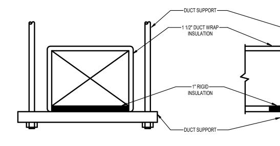
NOTES: 1. PROVIDE 1" RIGID INSULATION BOARD AT EACH DUCT HANGER. INSTALL DUCT WRAP INSULATION AROUND RIGID INSULATION BOARD.
