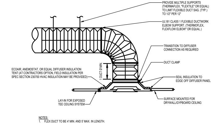
2. CONTRACTOR HAS THE OPTION OF INSTALLING AN INSULATED SHEET METAL TEE WITH CAP IN LIEU OF FLEX FLOW ELBOW.
