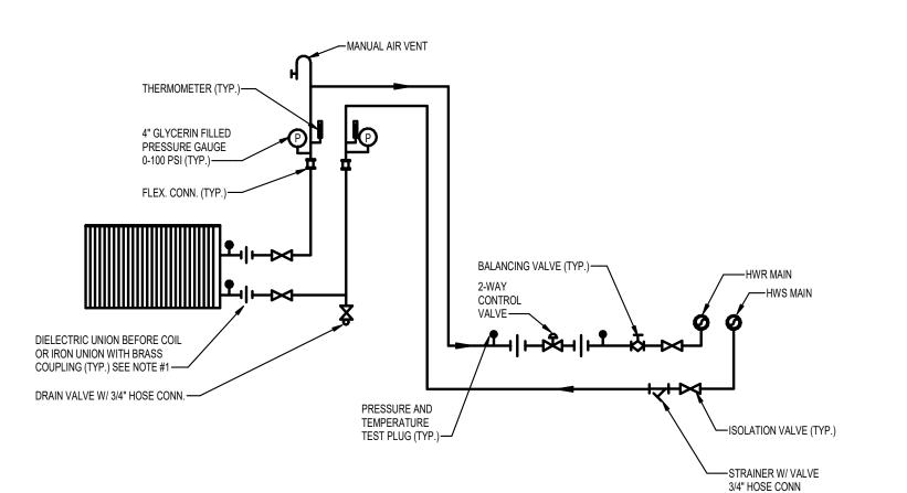
NOTES: 1. ARRANGE PIPING AND UNIONS TO ALLOW FOR COIL PULL. 2. DETAIL MAY NOT INDICATE EXACT NUMBER OF COIL CONNECTIONS. 3. PIPE HANGERS SHALL SUPPORT PIPING INDEPENDANTLY OF COIL.
