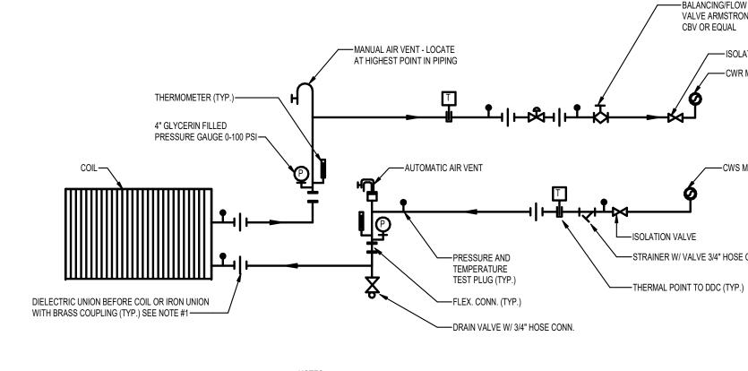
NOTES: 1. ARRANGE PIPING AND UNIONS TO ALLOW FOR COIL PULL. 2. DETAIL MAY NOT INDICATE EXACT NUMBER OF COIL CONNECTIONS
