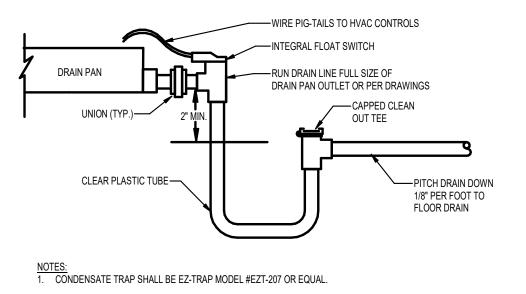
2. FLOAT SWITCH SHALL BE WIRED TO SHUT-DOWN UNIT AND ALARM AT THE BMS IF DRAIN LINE BECOMES CLOGGED.
