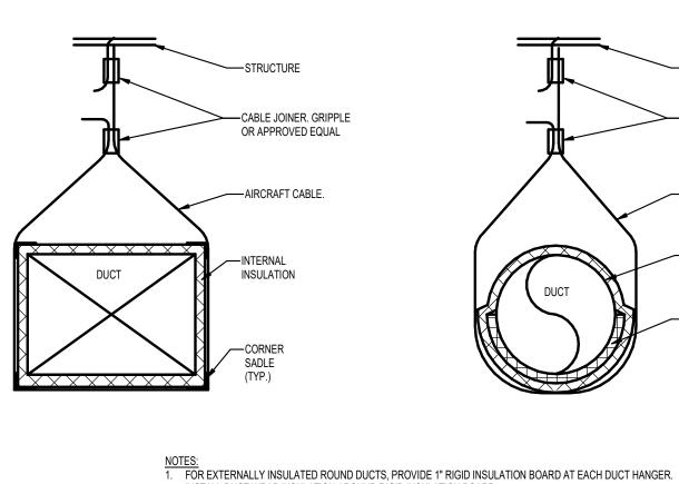
INSTALL DUCT WRAP INSULATION AROUND RIGID INSULATION BOARD. 2. FOR INTERNALLY INSULATED RECTANGULAR DUCTS, PROVIDE CORNER SADLES.
