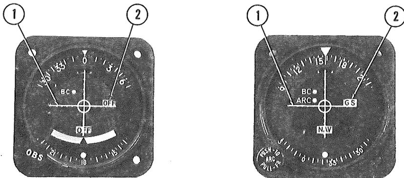
1. GLIDE SLOPE DEVIATION POINTER - Indicates deviation from normal glide slope.
