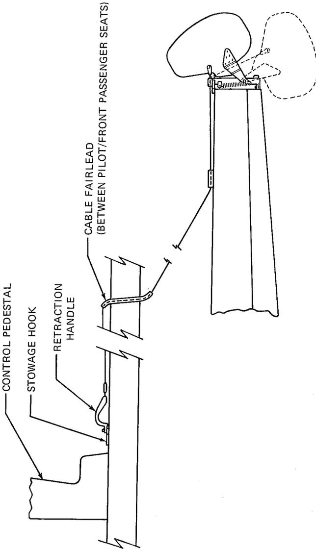
Figure 15. Water Rudder Retraction System
