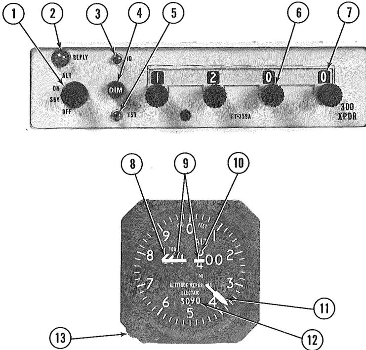
1. **FUNCTION SWITCH** - Controls application of power and selects transponder operating mode, as follows:
