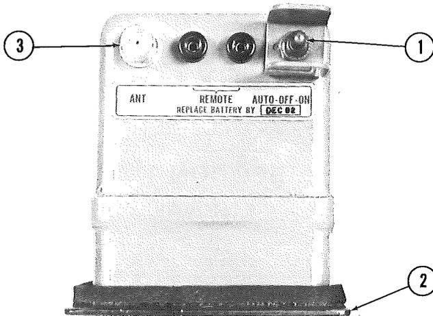
1. FUNCTION SELECTOR SWITCH (3-position toggle switch):
