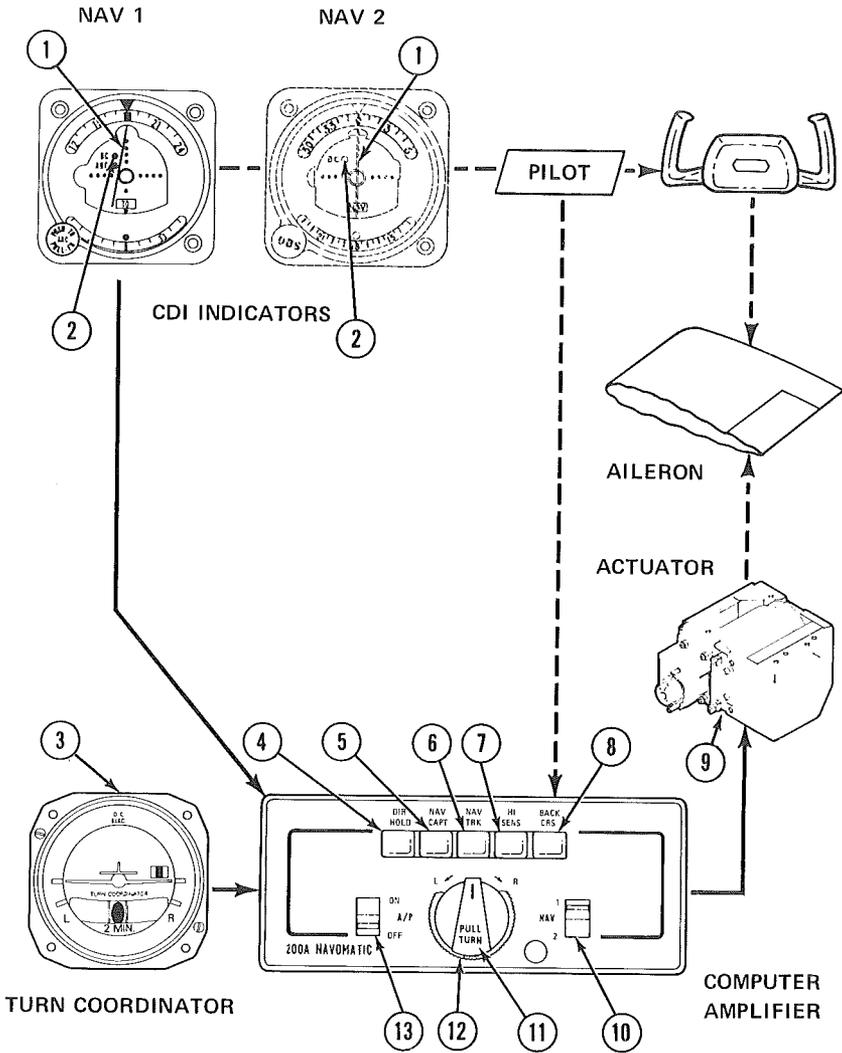
Figure 1. Cessna 200A Autopilot, Operating Controls and Indicators
