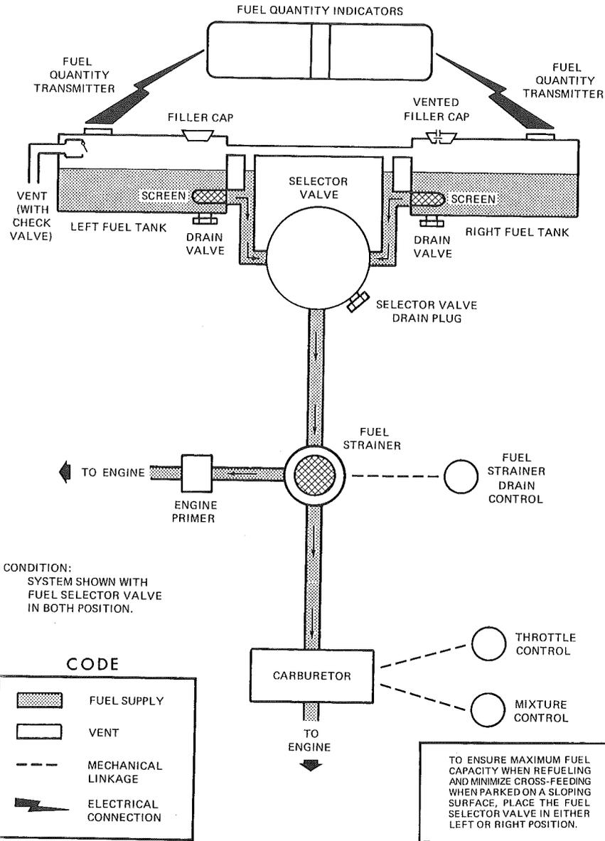
Figure 7-6. Fuel System (Standard and Long Range)
