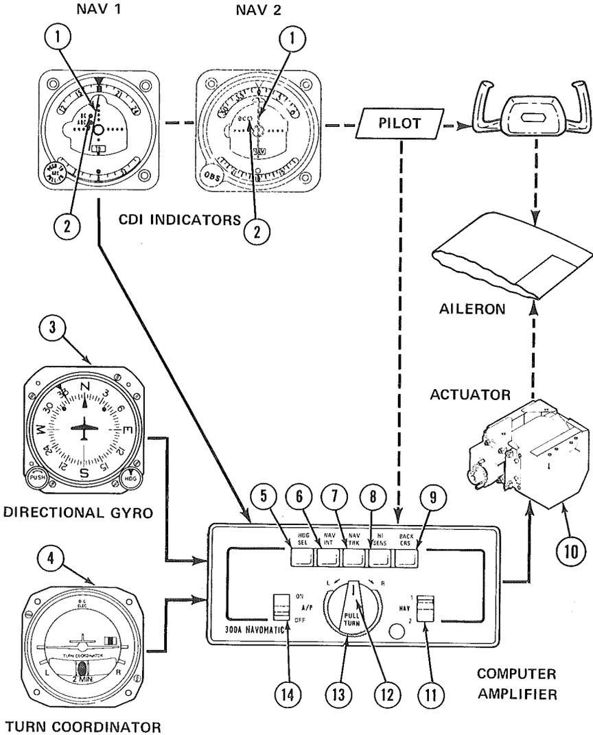
Figure 1. Cessna 300A Autopilot, Operating Controls and Indicators
