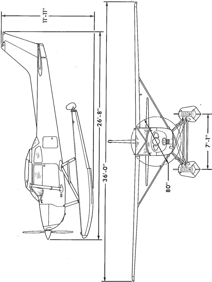
Figure 1. Three View (Sheet 1 of 2)
