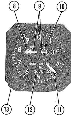
Figure 1. Cessna 400 Transponder and Encoding Altimeter
