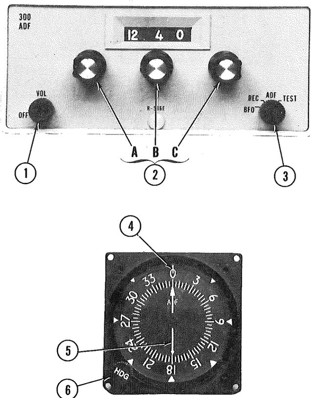
1. OFF/VOL CONTROL - Controls primary power and audio output level. Clockwise rotation from OFF position applies primary power to receiver; further clockwise rotation increases audio level.
