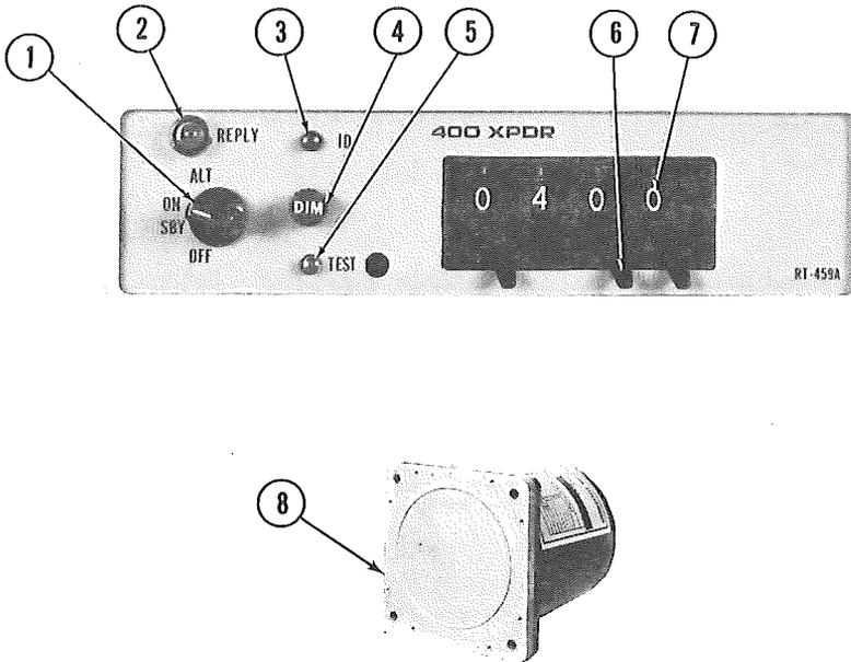
1. **FUNCTION SWITCH** - Controls application of power and selects transponder operating mode as follows:
