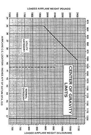
Figure 6-8. Center of Gravity Limits
