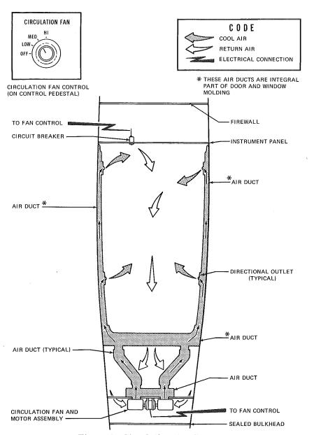
Figure 1. Circulation Fan System
