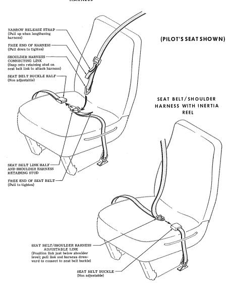
Figure 7-4. Seat Belts and Shoulder Harnesses
