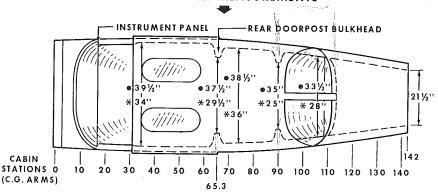
Figure 6-4. Internal Cabin Dimensions
