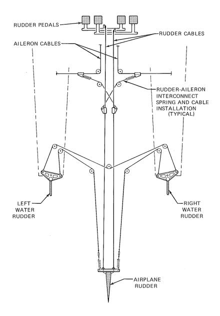
Figure 16. Water Rudder Steering System
