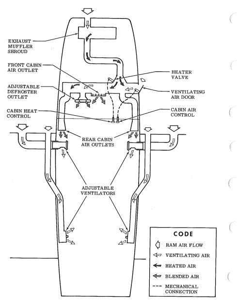
Figure 7-8. Cabin Heating, Ventilating, and Defrosting System
