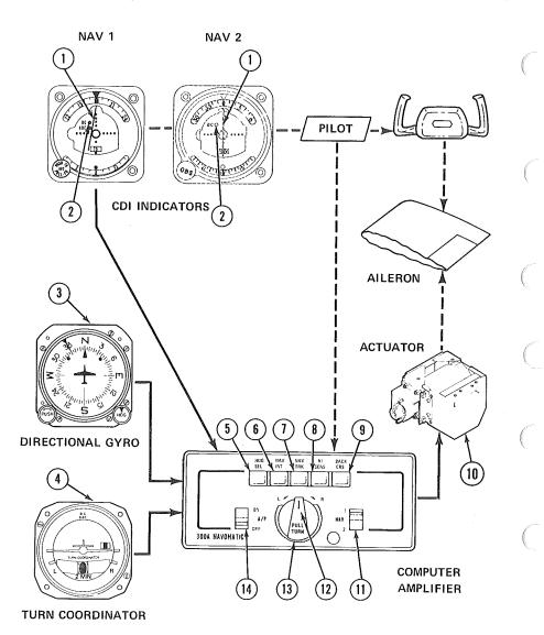
Figure 1. Cessna 300A Autopilot, Operating Controls and Indicators (Sheet 1 of 2)
