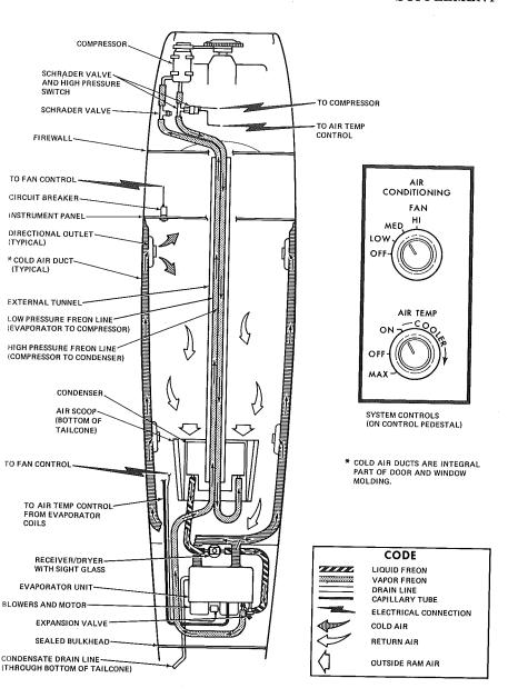
Figure 1. Air Conditioning System
