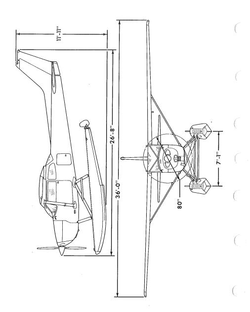
Figure 1. Three View (Sheet 1 of 2)
