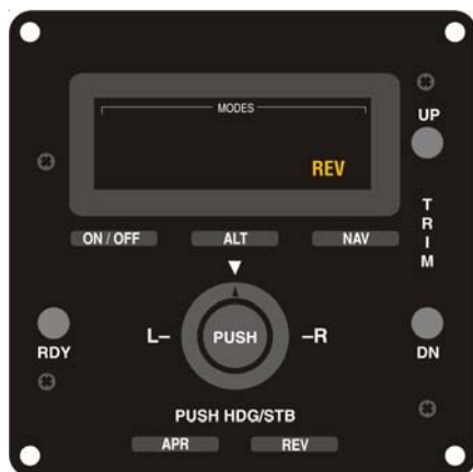
Fig. 2-21. AP Display, REV Mode Engaged (System Fifty)
