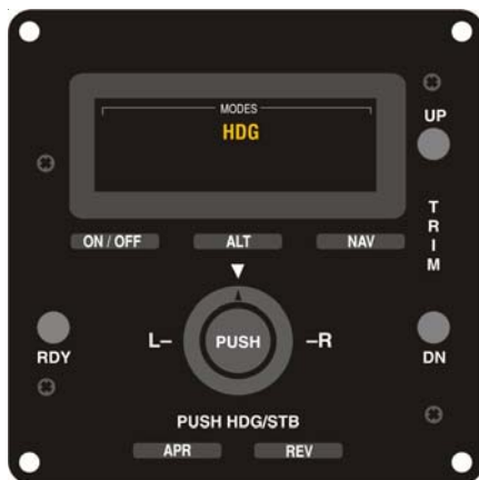
Fig. 2-18. AP Display, HDG Mode Engaged (System Fifty)
