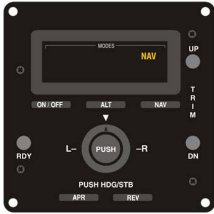
Fig. 2-19. AP Display, NAV Mode Engaged (System Fifty)
