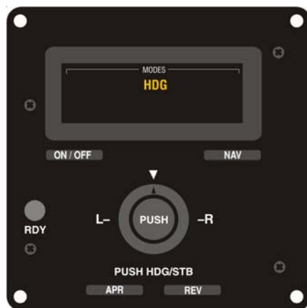
Fig. 2-6. AP Display, HDG Mode Engaged (System Forty)
