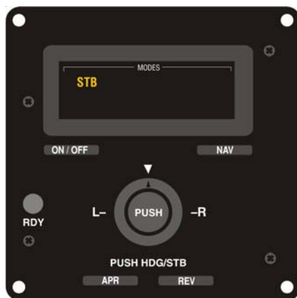
Fig. 2-5. AP Display, STB Mode Engaged (System Forty)
