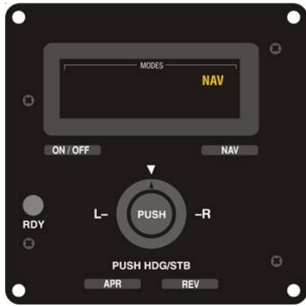
Fig. 2-7. AP Display, NAV Mode Engaged (System Forty)
