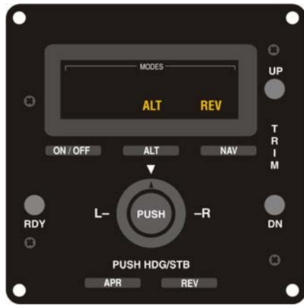
Fig. 2-22. AP Display, REV and ALT HOLD Modes Engaged (System Fifty)
