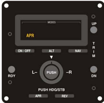
Fig. 2-20. AP Display, APR Mode Engaged (System Fifty)
