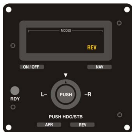
Fig. 2-9. AP Display, REV Mode Engaged (System Forty)
