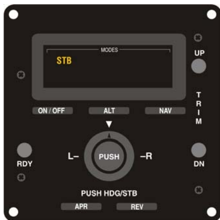
Fig. 2-17. AP Display, STB Mode Engaged (System Fifty)
