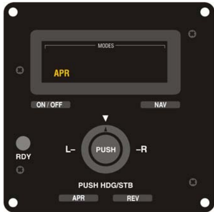
Fig. 2-8. AP Display, APR Mode Engaged (System Forty)
