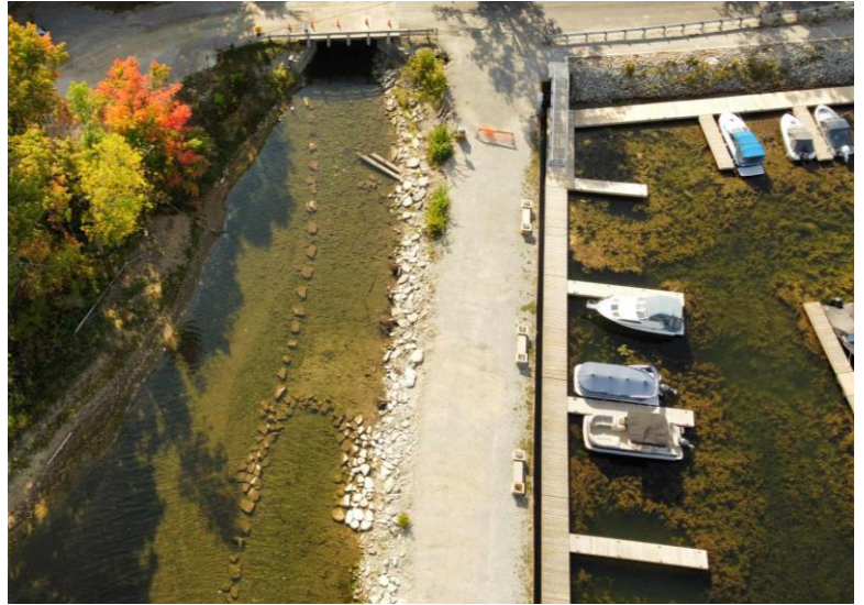
In imagery taken with Liam's drone, we get an overhead view of KAG 180, clearly showing the line of boulders and rock weirs.
