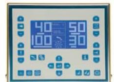
**If needed this controller can be remote controlled by a PC through a CAN-BUS. All the parameters are displayed on the graphical display. Additional Software and CAN-BUS extension card for a PC needed.**
