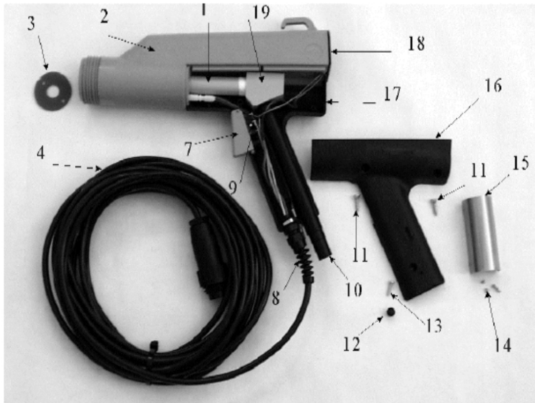
Illustration 6 Overview of a disassembled MG801
