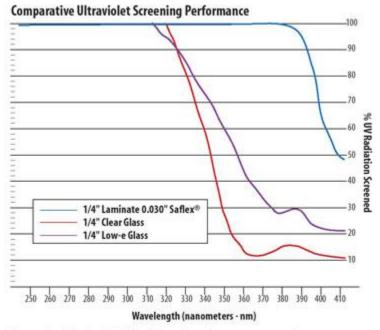
UV screening defined as the ability of the configuration to screen greater than 99% of UV radiation to 380nm wave length.
