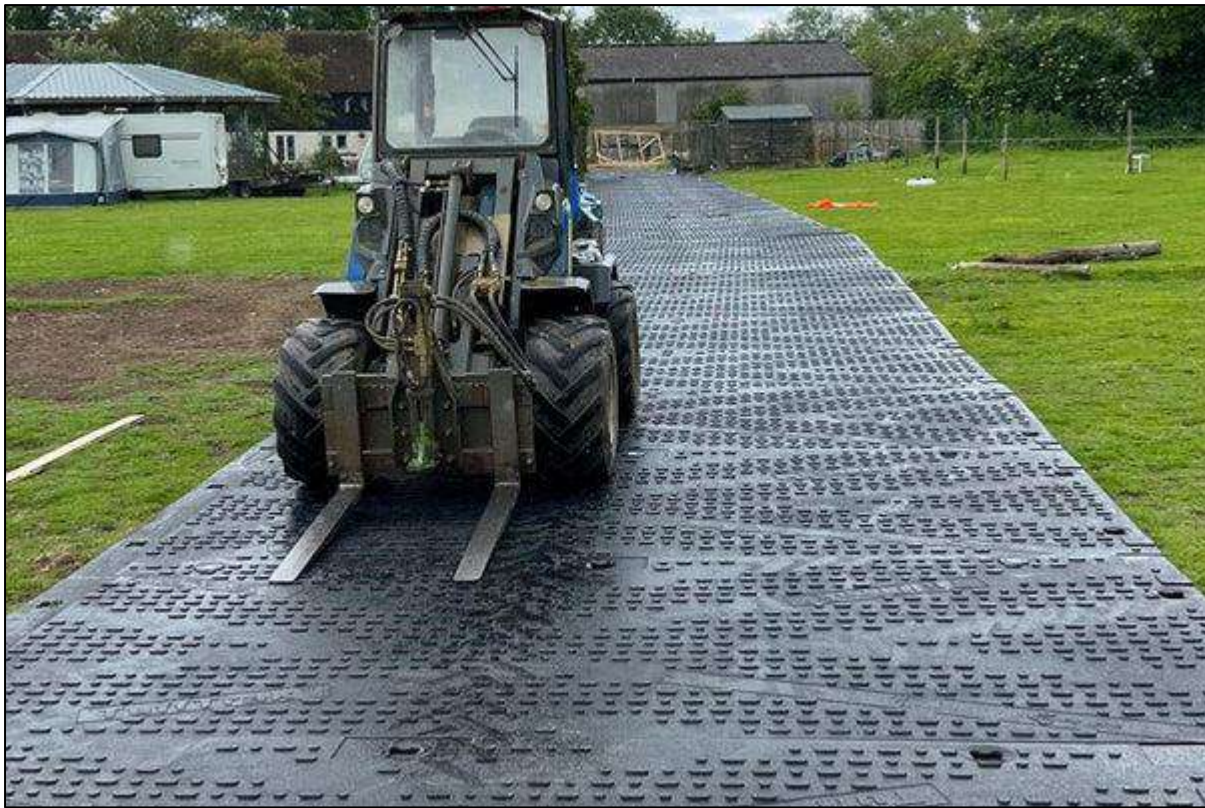
Figure 8 - Example Rubber Temporary Trackway
