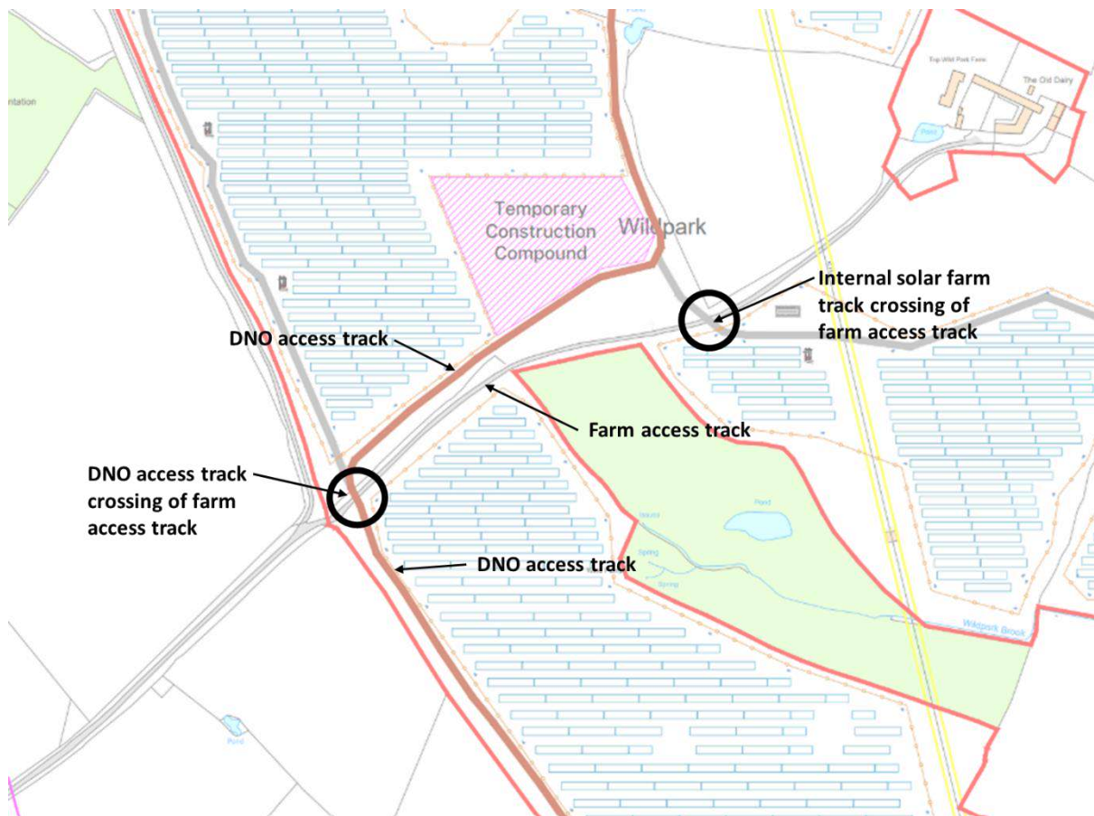
Figure 13 – DNO Access Track Crossing
