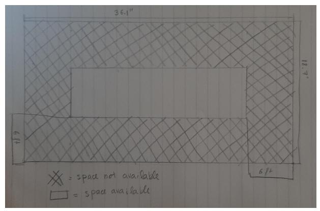
In this image the space of the playground with dimensions is drawn. The original dimensions are shown, as well as the ones after the 6 feet distance constraint.
