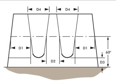
Figure 23. Minimum Clearances for Single-Axis Swings
