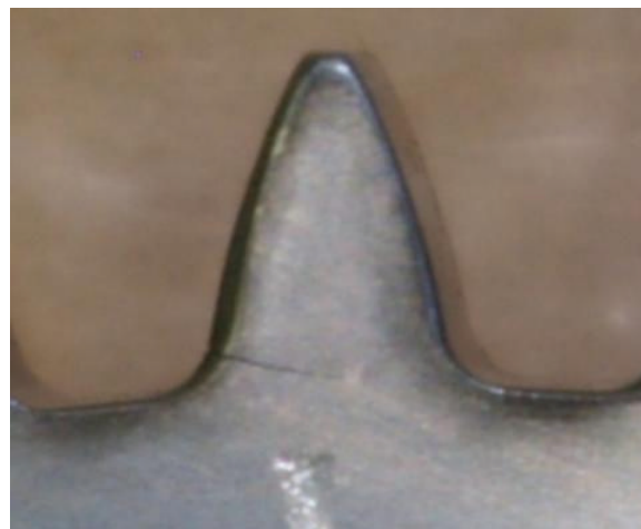
Figure 10: Typical fatigue crack generated by cyclic tooth bending.
