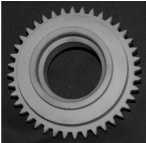
Figure 1. Carburized and quench hardened spur gear.
