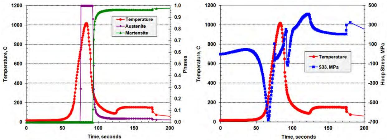
Figure 7 Temperature, phase and hoop stress histories experienced at the mid-length bore location of the tube. (N.B. Process is not completed until 475 seconds.)
