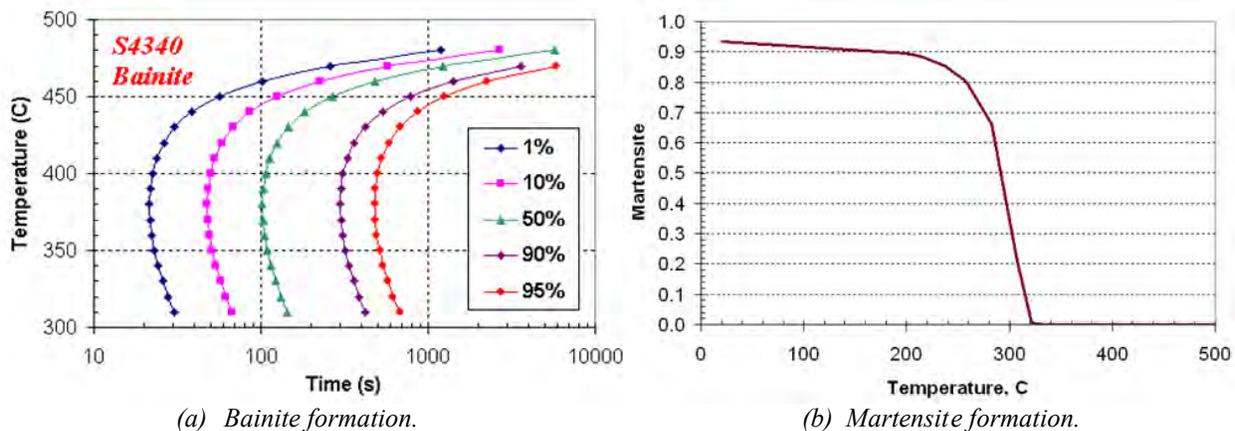
Figure 2 Kinetics data for 4340 steel.
