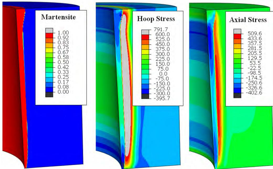
Figure 6 Final martensite, hoop and axial stress profiles predicted by DANTE. (Stress is MPa)
