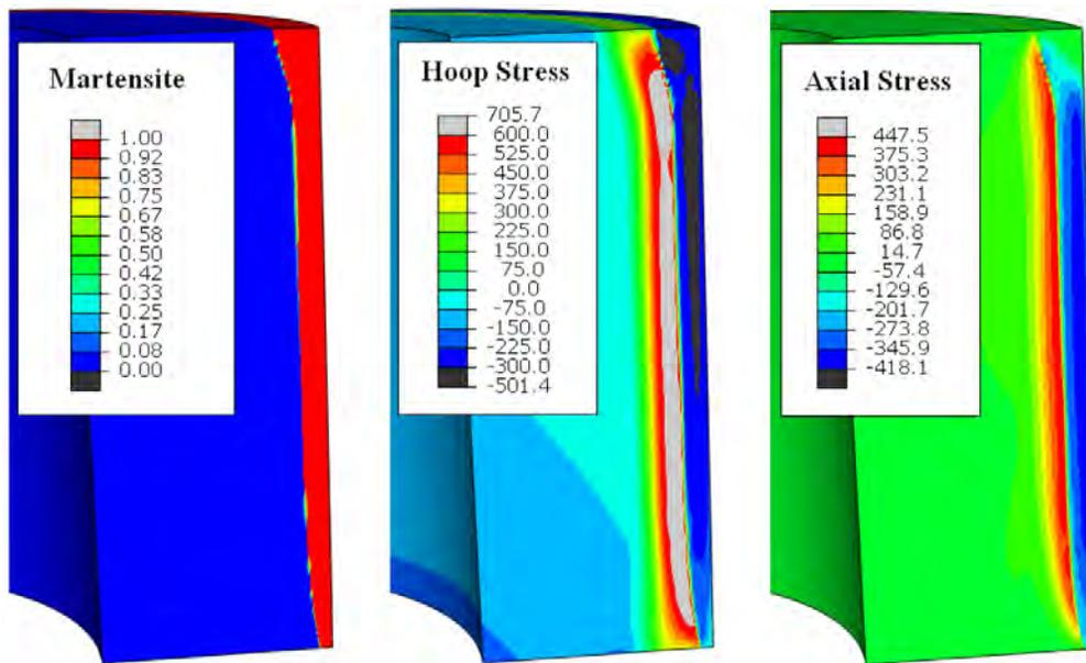
Figure 10 Final martensite, hoop and axial stress profile predictions for OD scan hardening.
