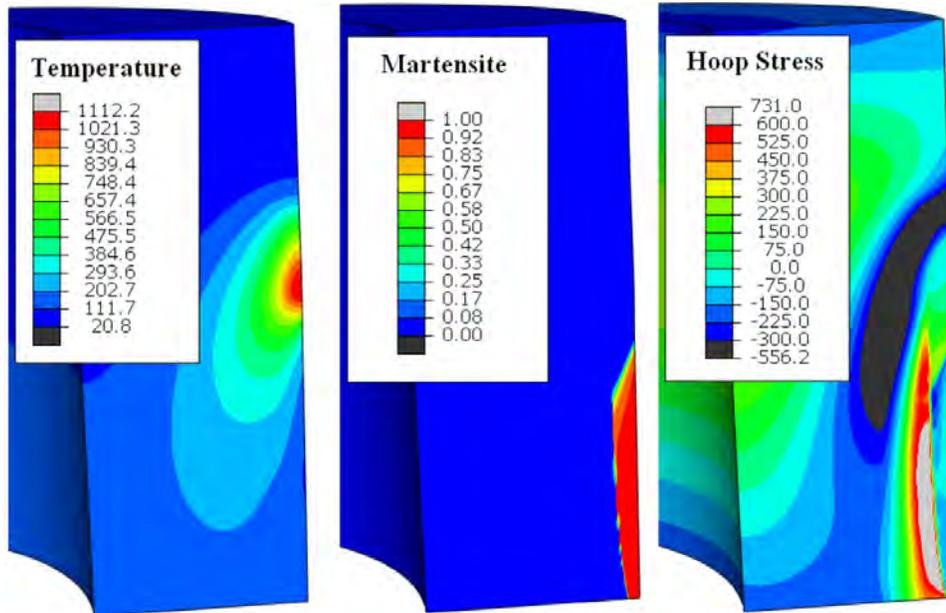
Figure 8 Predicted temperature, martensite and hoop stress profiles at roughly midway through the OD scan hardening process. (Stress is MPa)
