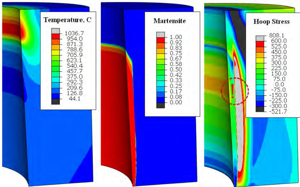
Figure 5 Temperature, martensite and hoop stress profiles predicted by DANTE nearing completion of the process. (Stress is MPa)
