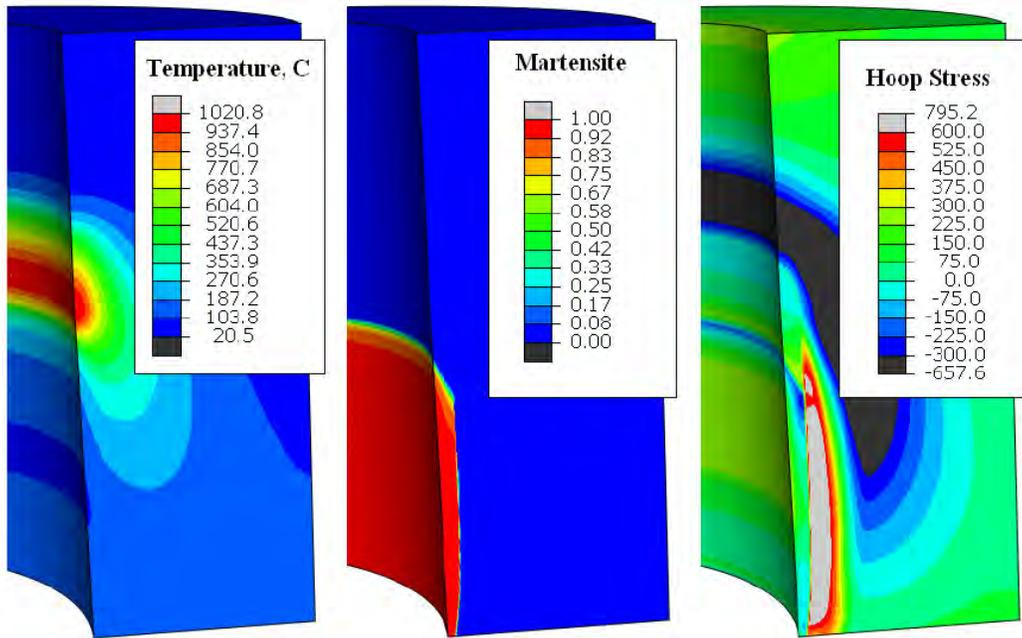
Figure 4 Temperature, martensite and hoop stress profiles predicted by DANTE at roughly midway through the ID scan hardening process. (Stress is MPa)
