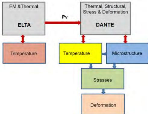
Figure 1 Calculations performed by Elta and DANTE and passing of data between the programs.
