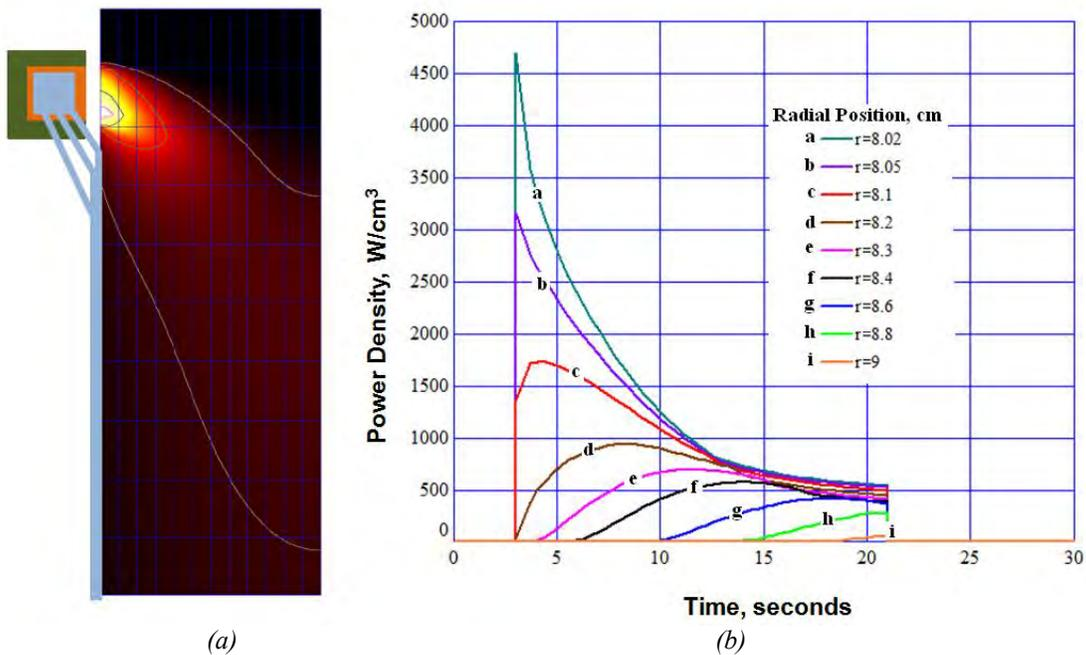
(a) Schematic of induction hardening and spray quench.
