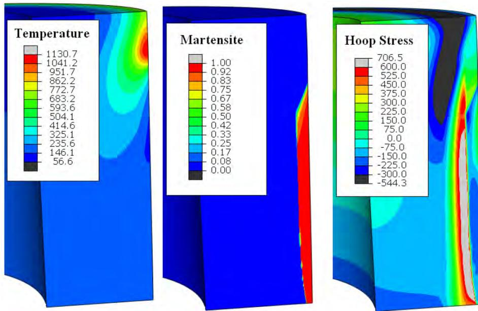
Figure 9 Temperature, martensite and hoop stress profiles predicted near completion of the heating step of the scan hardening process. (Stress is MPa)
