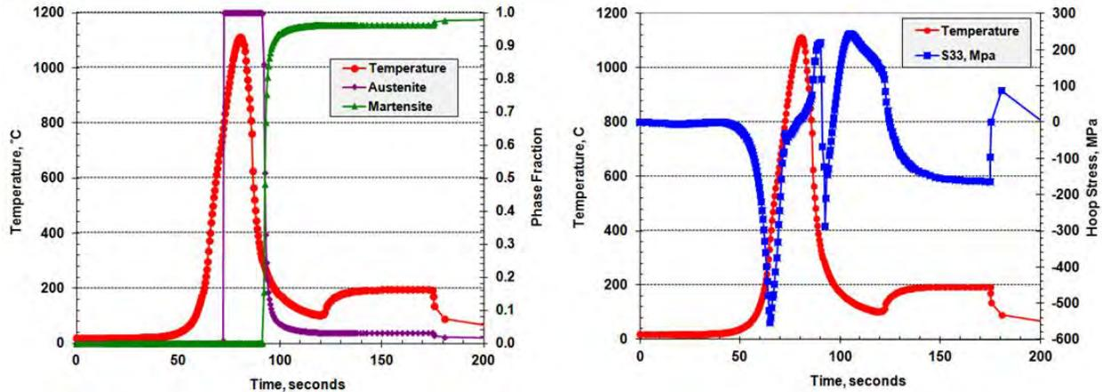
Figure 11 Temperature, phase and hoop stress histories experienced at the mid-length bore location of the tube. (N.B. Process is not completed until 475 seconds.)
