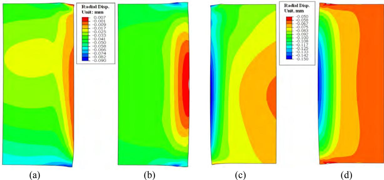
Figure 12 Radial displacement distribution at the end of cooling for OD and ID treatment.
