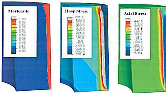
Figure 6: Distribution of martensite, hoop and axial stresses at the end of OD treatment.
