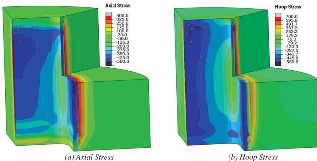
Figure 5: Residual stress distributions produced by the innovative induction hardening process.
