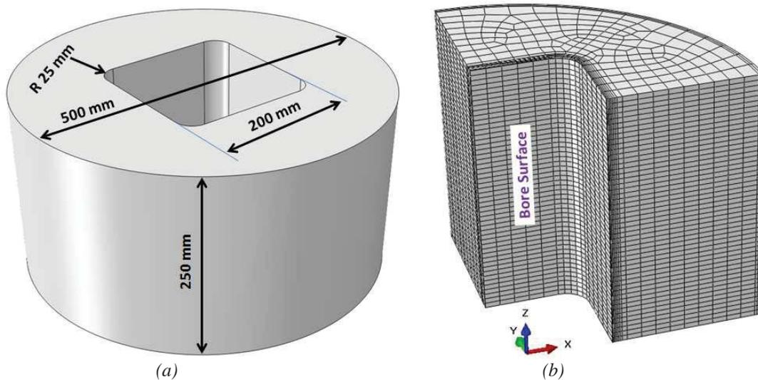
Figure 1: (a) Geometry of the generic coupler, and (b) finite element mesh.
