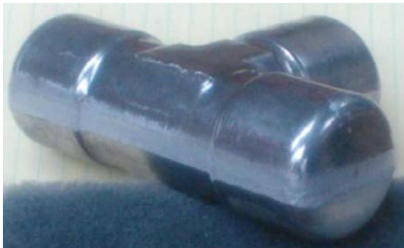
Figure 5. “Tee” forging of 7075 aluminum.
