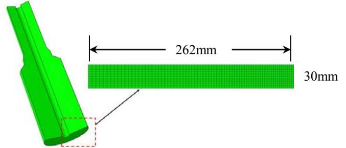
Figure 3: 2-D mesh slice through the roll body for the DANTE models.
