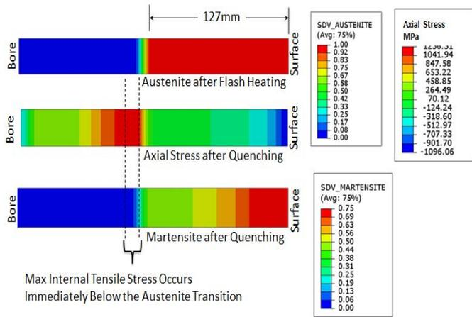
Figure 9: Composite contour plot showing flash heated austenitizing depth relative to the post quenching axial stress and martensite phase fraction profiles for the roll austenitized to 127mm depth.
