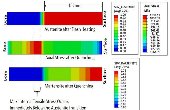
Figure 8: Composite contour plot showing flash heated austenitizing depth relative to the post quenching axial stress and martensite phase fraction profiles for the roll austenitized to 152mm depth.
