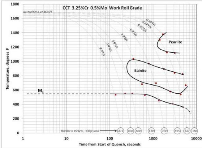
Figure 1: Experimentally determined continuous cooling transformation diagram for the 3.25% Cr alloy roll steel.
