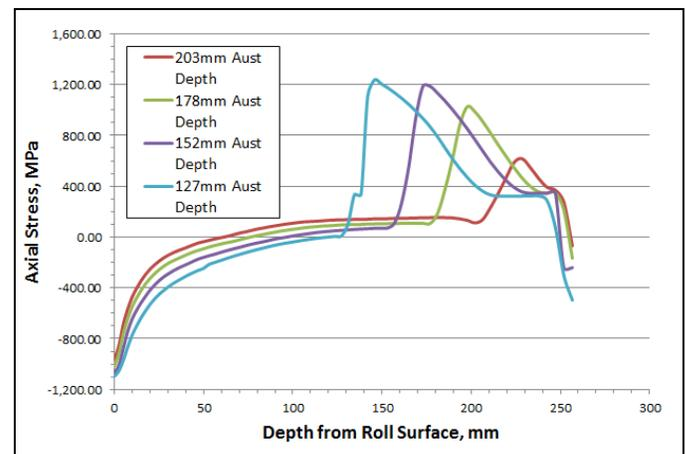
Figure 4: Comparative axial stress profiles for the roll body, showing the effect of austenitizing depth.
