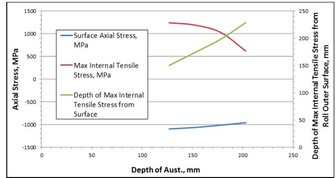
Figure 10: Composite contour plot showing flash heated austenitizing depth relative to the post quenching axial stress and martensite phase fraction profiles for the roll austenitized to 127mm depth.
