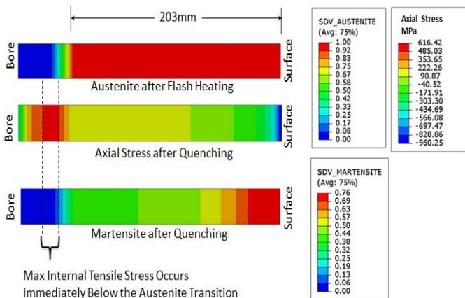
Figure 6: Composite contour plot showing flash heated austenitizing depth relative to the post quenching axial stress and martensite phase fraction profiles for the roll austenitized to 203mm depth.
