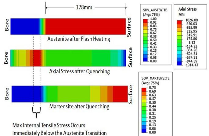
Figure 7: Composite contour plot showing flash heated austenitizing depth relative to the post quenching axial stress and martensite phase fraction profiles for the roll austenitized to 178mm depth.
