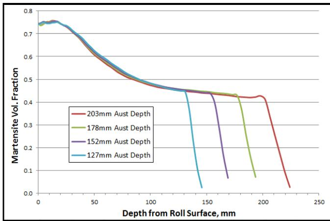
Figure 5: Comparative martensite volume fraction profiles for the roll body, showing the effect of austenitizing depth. Compare with the stress plot in Figure 4.
