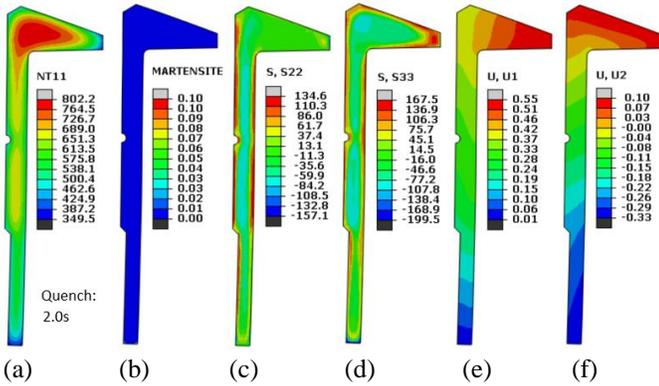
Figure 9. Modeling results at 2.0 seconds of immersion quench. a) temperature, b) martensite, c) axial stress, d) circumferential stress, e) radial displacement, and f) axial displacement.
