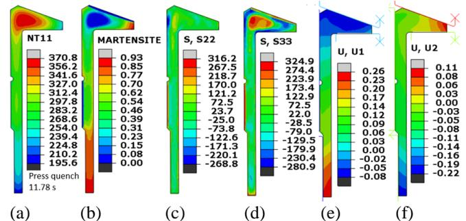
Figure 16. Modeling results at 11.78 seconds of press quench. a) temperature, b) martensite, c) axial stress, d) circumferential stress, e) radial displacement, and f) axial displacement.
