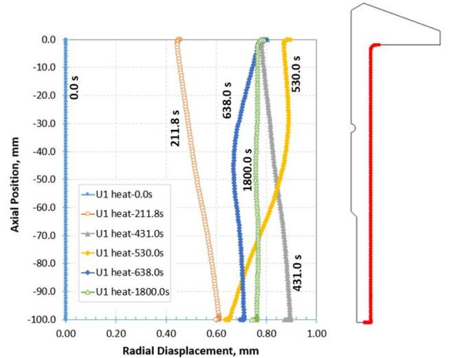
Figure 7. Effect of thermal expansion and austenitic phase transformation on the radial displacement of the gear wall during heating.
