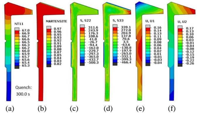
Figure 11. Modeling results after cooling the gear to the oil temperature using immersion quench. a) temperature, b) martensite, c) axial stress, d) circumferential stress, e) radial displacement, and f) axial displacement.
