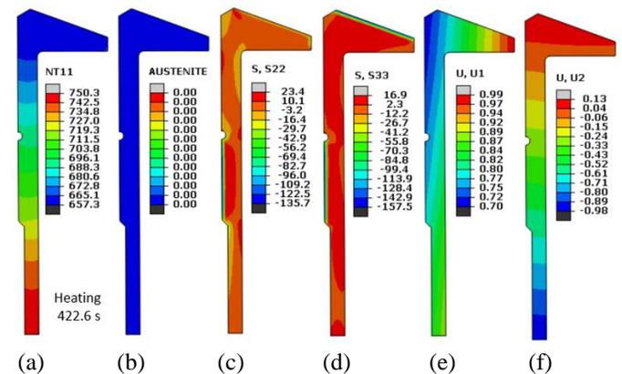
Figure 4. Modeling results during heating at 422.6 seconds. a) temperature, b) austenite, c) axial stress, d) circumferential stress, e) radial displacement, and f) axial displacement.
