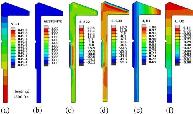
Figure 6. Modeling results at the end of heating. a) temperature, b) austenite, c) axial stress, d) circumferential stress, e) radial displacement, and f) axial displacement.
