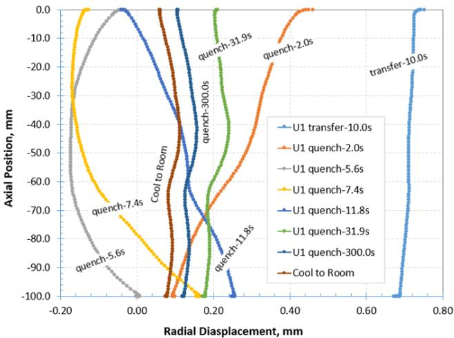
Figure 18. Effect of thermal shrinkage and martensitic phase transformation on the radial displacement of the gear wall during press quench process.
