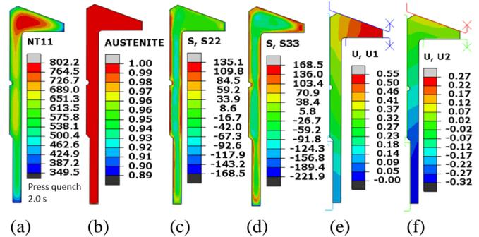
Figure 15. Modeling results at 2.0 seconds of press quench. a) temperature, b) martensite, c) axial stress, d) circumferential stress, e) radial displacement, and f) axial displacement.
