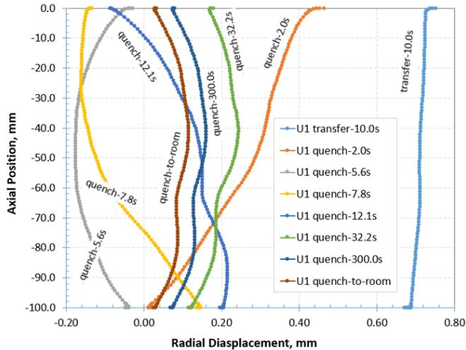
Figure 13. Effect of thermal shrinkage and martensitic phase transformation on the radial displacement of the gear wall during immersion quench process.
