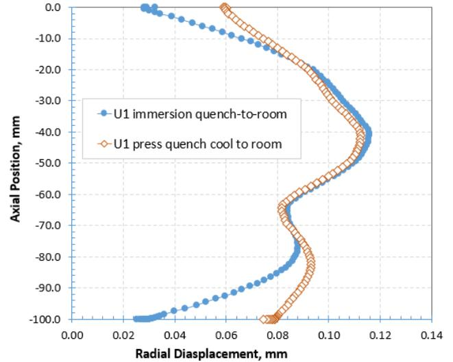
Figure 19. Comparison of predicted radial displacements of the gear wall between the press quench and immersion quench processes.
