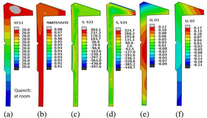
Figure 12. Modeling results after cooling the gear to room temperature using immersion quench. a) temperature, b) martensite, c) axial stress, d) circumferential stress, e) radial displacement, and f) axial displacement.
