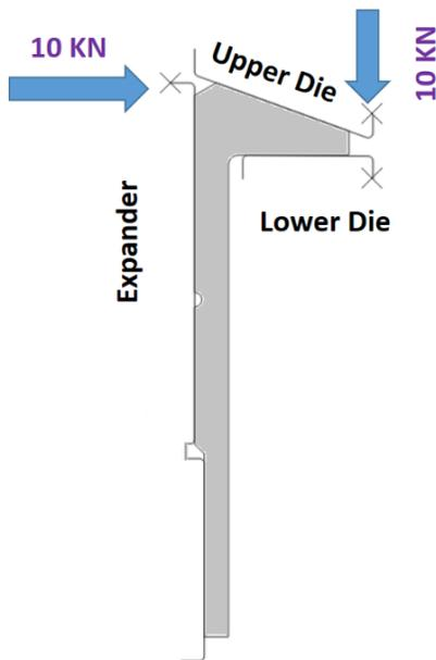
Figure 14. Schematic tooling set up for press quench process modeling.
