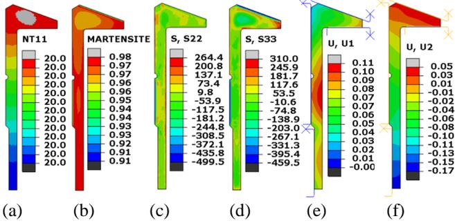
Figure 17. Modeling results after cooling the gear to room temperature using press quench. a) temperature, b) martensite, c) axial stress, d) circumferential stress, e) radial displacement, and f) axial displacement.
