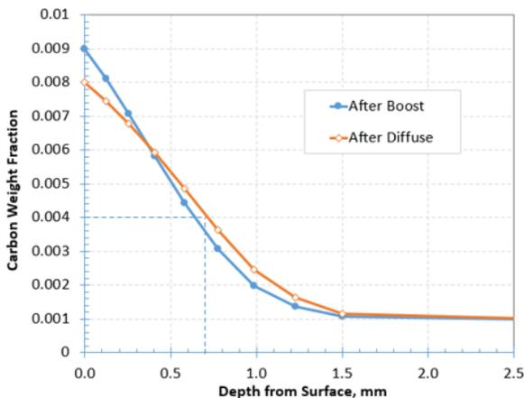
Figure 3. Carbon distributions in terms of depth after the boost and diffusion steps.
