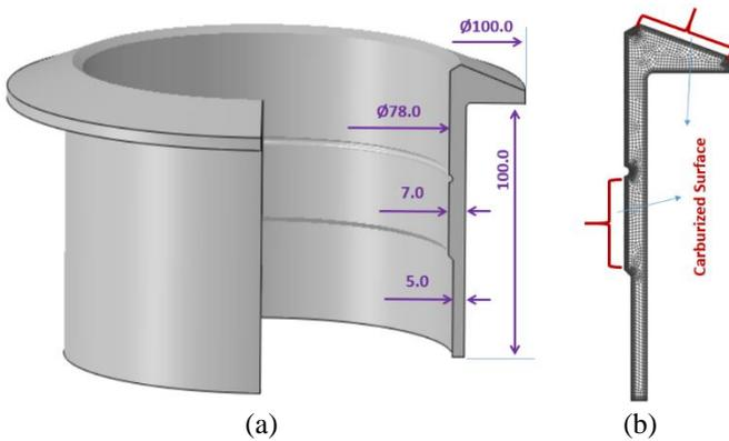
Figure 2. Simplified thin-wall bevel gear. a) CAD model and dimensions, and b) Finite element mesh.
