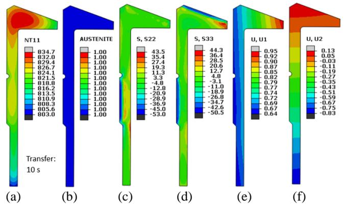
Figure 8. Modeling results at the end of the 10 second air transfer step. a) temperature, b) austenite, c) axial stress, d) circumferential stress, e) radial displacement, and f) axial displacement.
