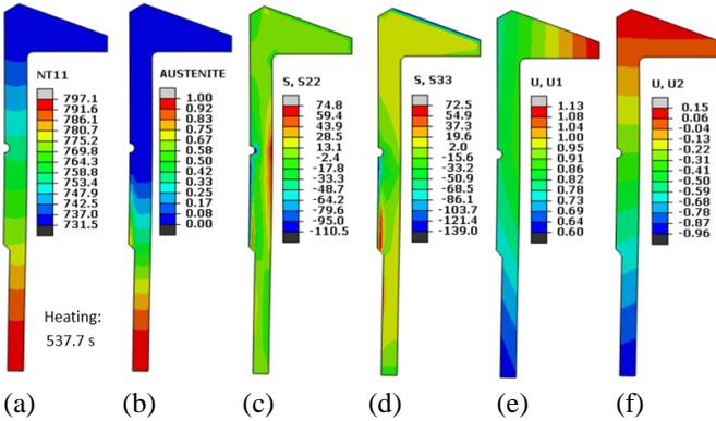
Figure 5. Modeling results during heating at 537.7 seconds. a) temperature, b) austenite, c) axial stress, d) circumferential stress, e) radial displacement, and f) axial displacement.
