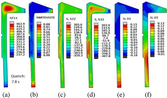
Figure 10. Modeling results at 7.8 seconds of immersion quench. a) temperature, b) martensite, c) axial stress, d) circumferential stress, e) radial displacement, and f) axial displacement.
