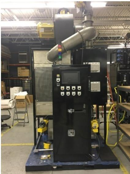
DANTE Solutions, in collaboration with Atmosphere Engineering and Akron Steel Treating, designed an innovative gas quenching unit to minimize component distortion during the hardening process. The DANTE Controlled Gas Quenching (DCGQ) unit is capable of quenching single components following a time-temperature schedule designed for a specific component and steel alloy using the DANTE software.
